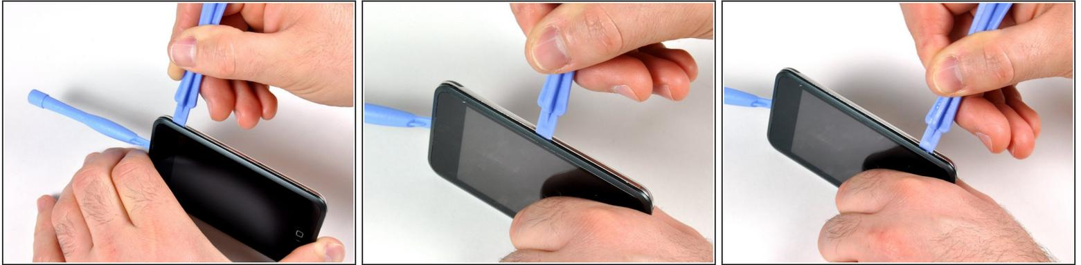
**i** There are seven interlocking retaining clips on each side of the iPod. The large plastic opening tool will be used to separate the front panel from the metal back of the iPod.
