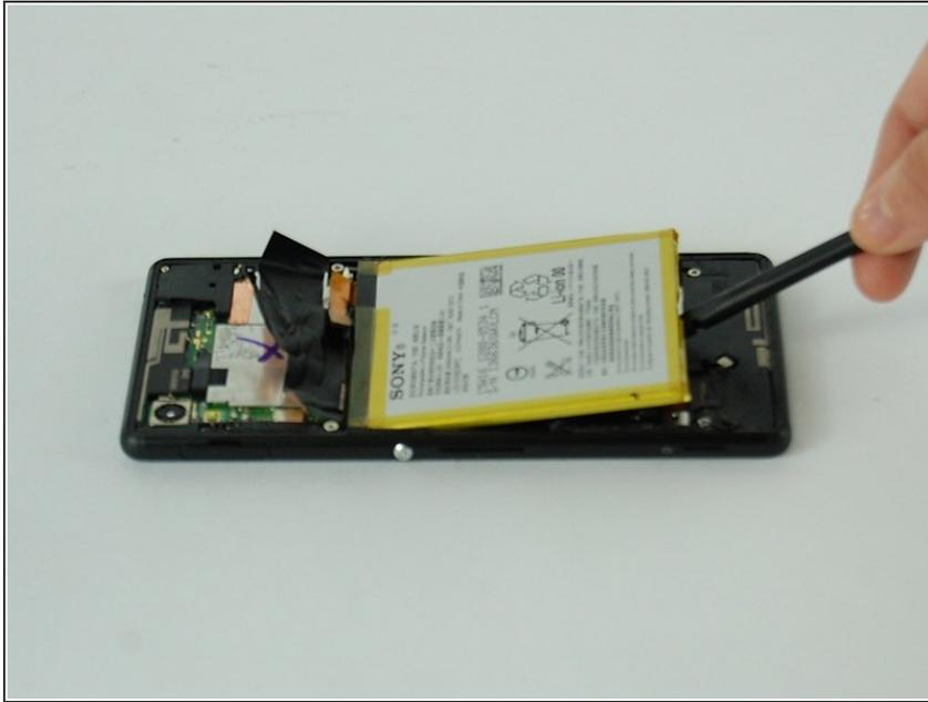
**⚠** Pry the battery from the phone with the nylon spudger. There is a small amount of adhesive underneath the battery, so a bit of force is required. The battery is malleable, so it is possible to dent the battery if too much force is applied in one spot.
