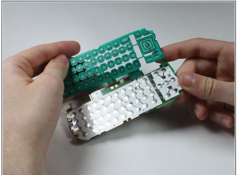
**i** The circuit board and the key board will be attached, as shown in the second picture.
