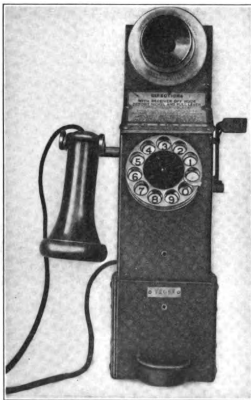
FIG. 83.—A combination telephone and coin collector for both local and toll-line service.
