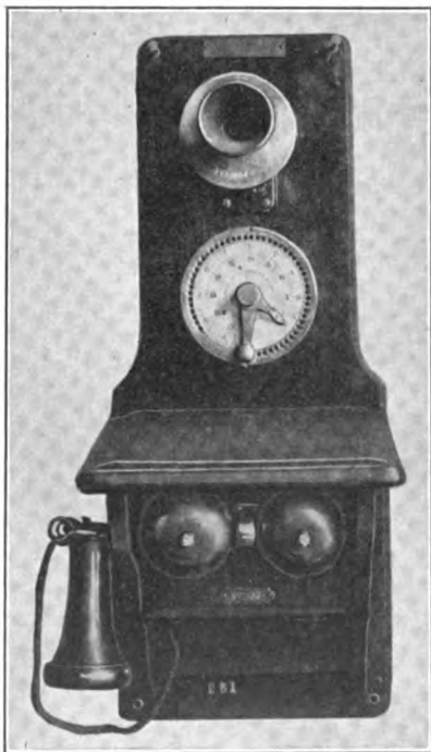
FIG. 88.—Wall telephone with later calling device.
