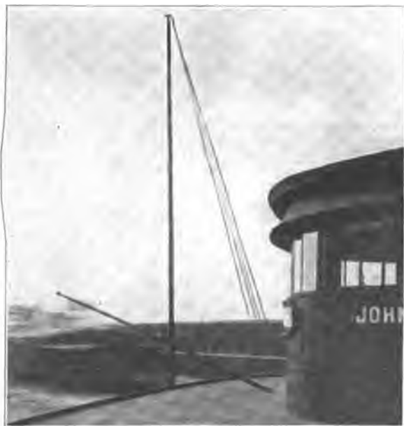
Upper Deck of John G. McCullough, Showing Aerial Wires Used in Collins System.
