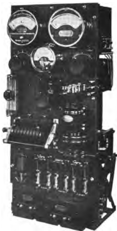
Fig. 250—Special Submarine Type Panel Transmitter (American Marconi Company).
