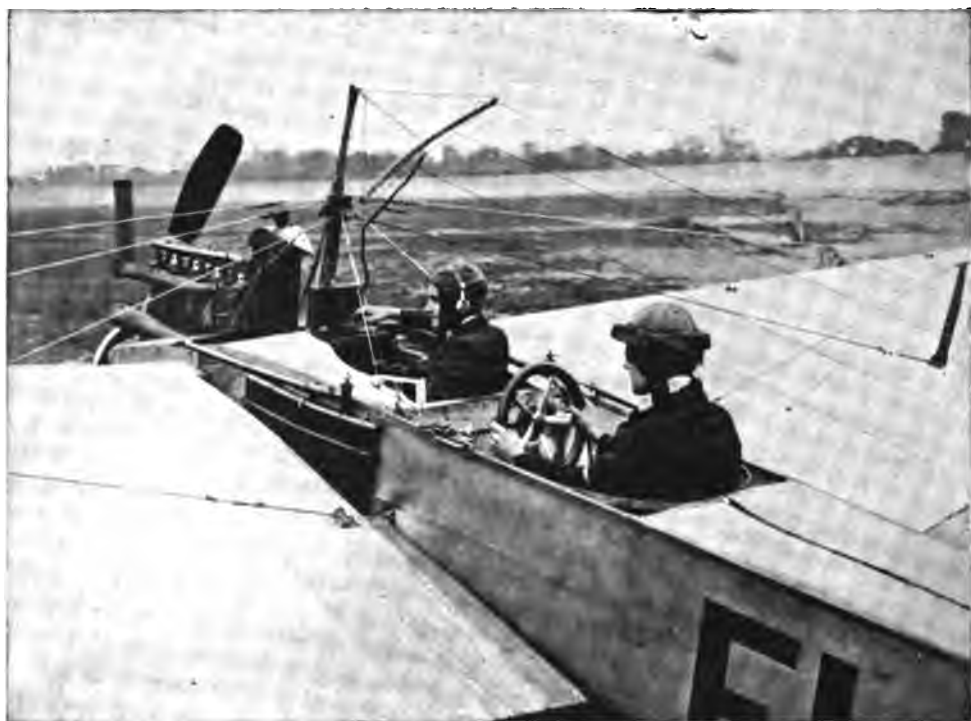
Fig. 325A—Scout Airplane Equipped With Wirel  s Apparatus.
