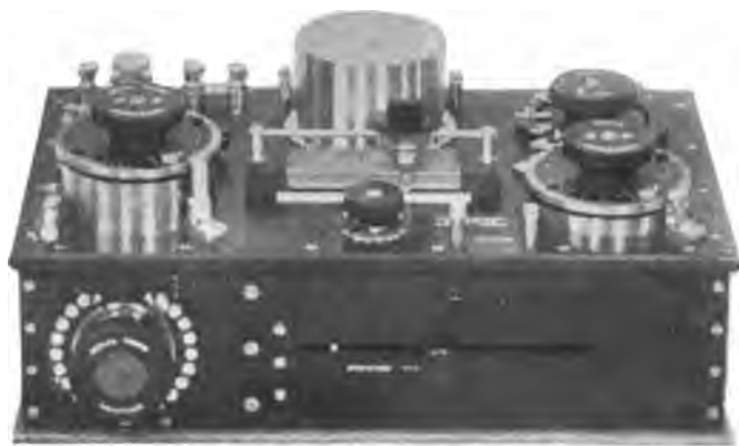
Fig. 177—Universal Crystal Receiver (English Marconi Company).
