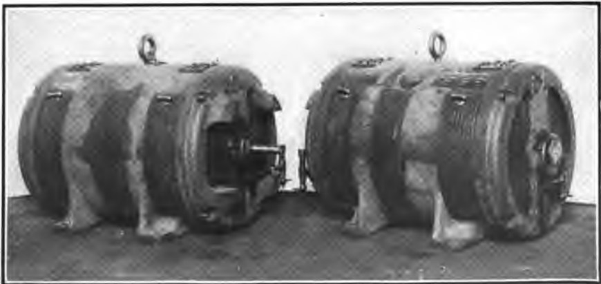
Fig. 67b—2 K. W. Crocker-Wheeler Motor Generator Assembled.
