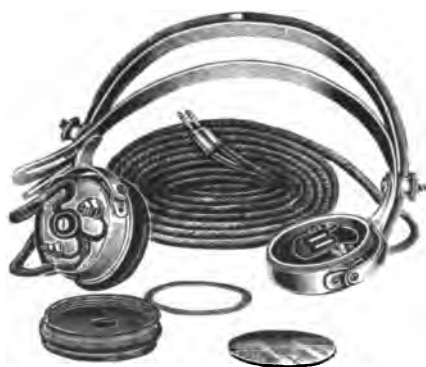
Fig. 194a—3 000-Ohm Head Telephone Receiver.
