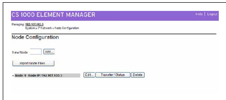
Figure 60 Adding a new node
