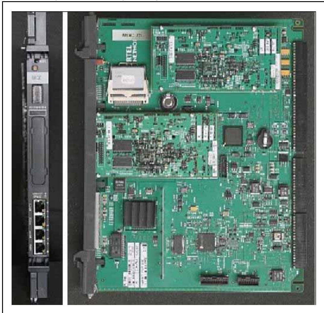
Figure 6 Media Gateway Controller card (NTDW60)
