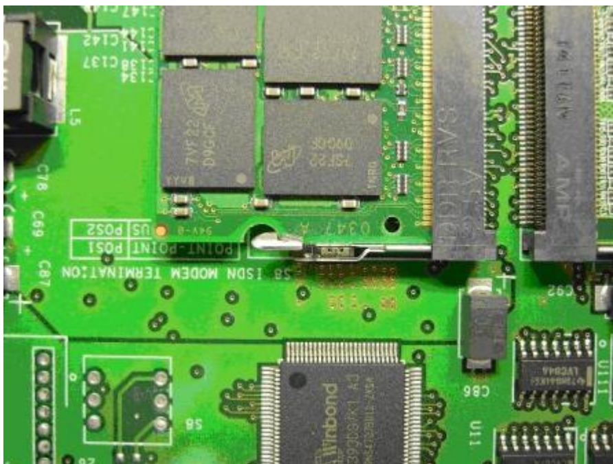
Figure 185: Fastening memory module in CP PM card
