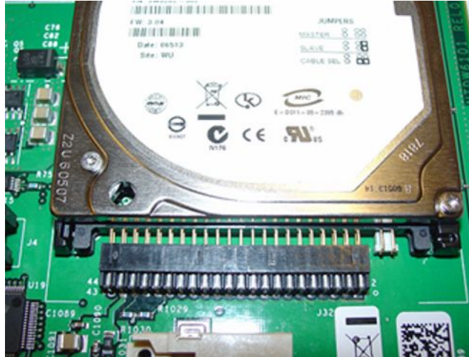
Figure 178: CP PM hard drive and connector J32
