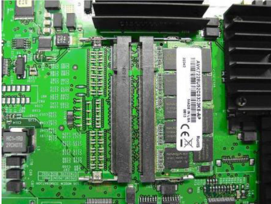
Figure 183: CP PM card with empty memory slot
