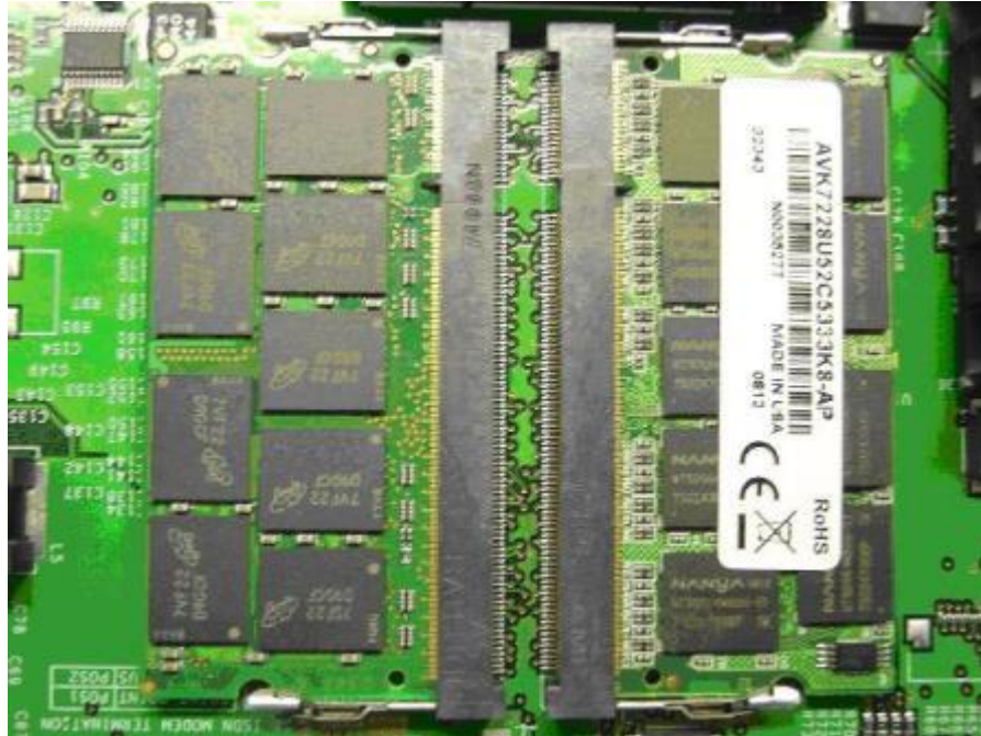
Figure 187: Correctly aligned memory module
