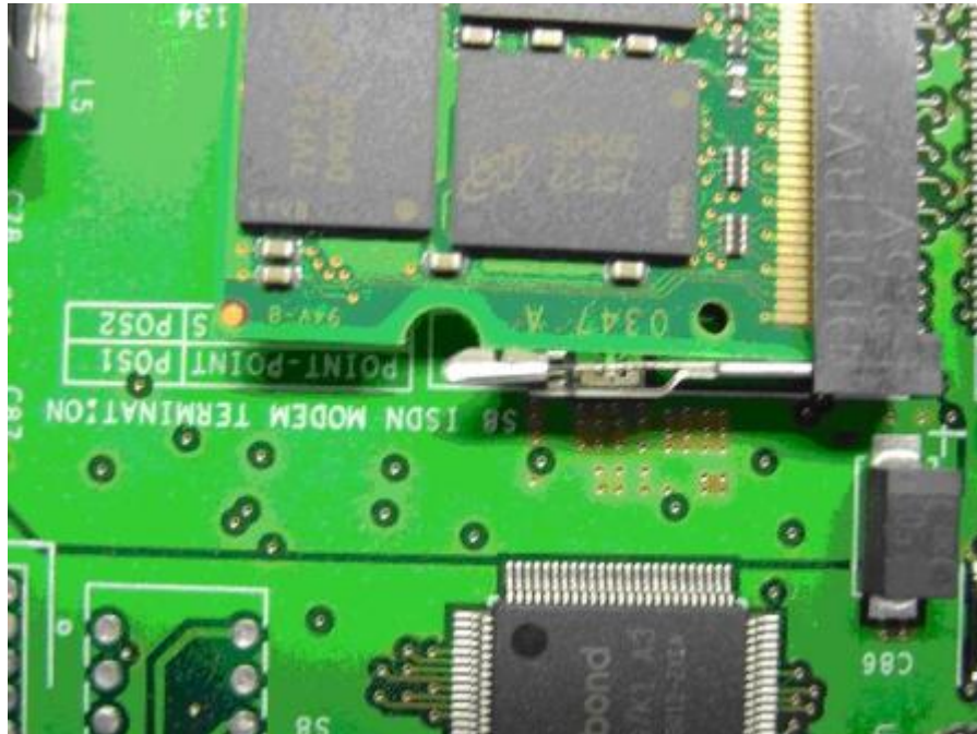
Figure 186: Incorrectly aligned memory module
