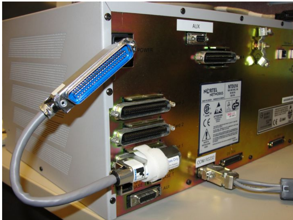
Figure 11: Connecting the surge suppression cable to the Media Gateway
