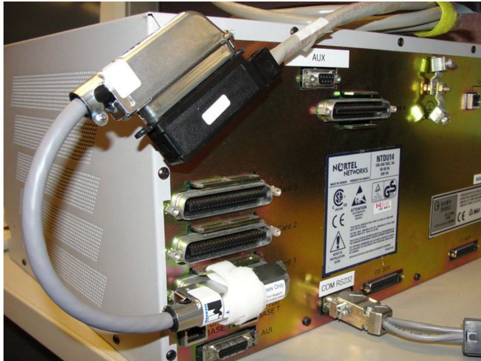
Figure 12: Connecting the surge suppression cable to the CS 1000 system MDF cable
