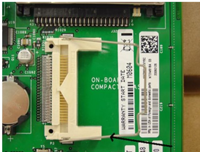
Figure 181: CP PM Signaling Server internal CF card retainer clip
