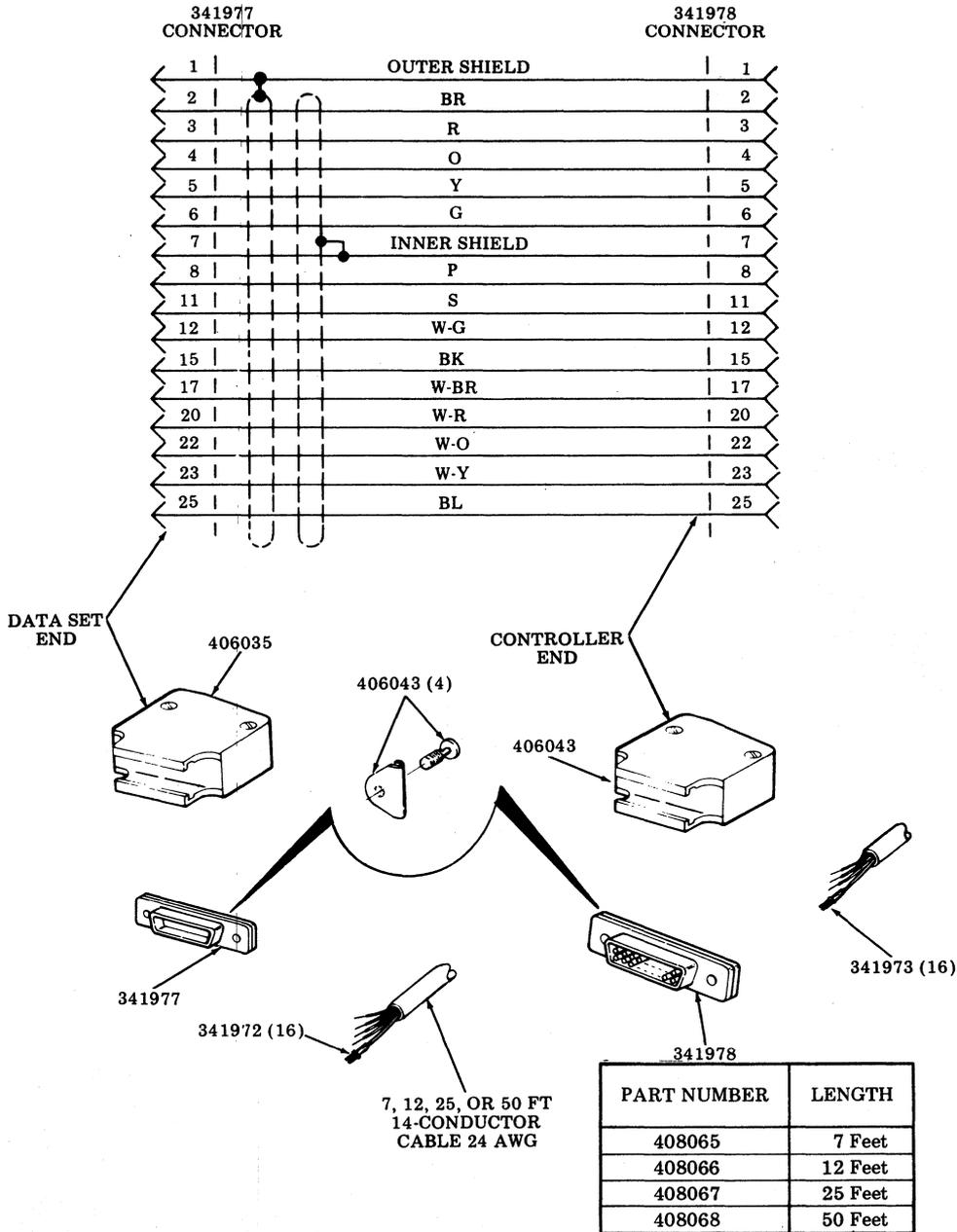
Fig. 8—Data Set Extension Cable Assemblies
