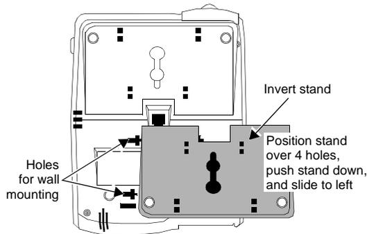
**Figure 7. Installing the Stand for Wall Mounting**
