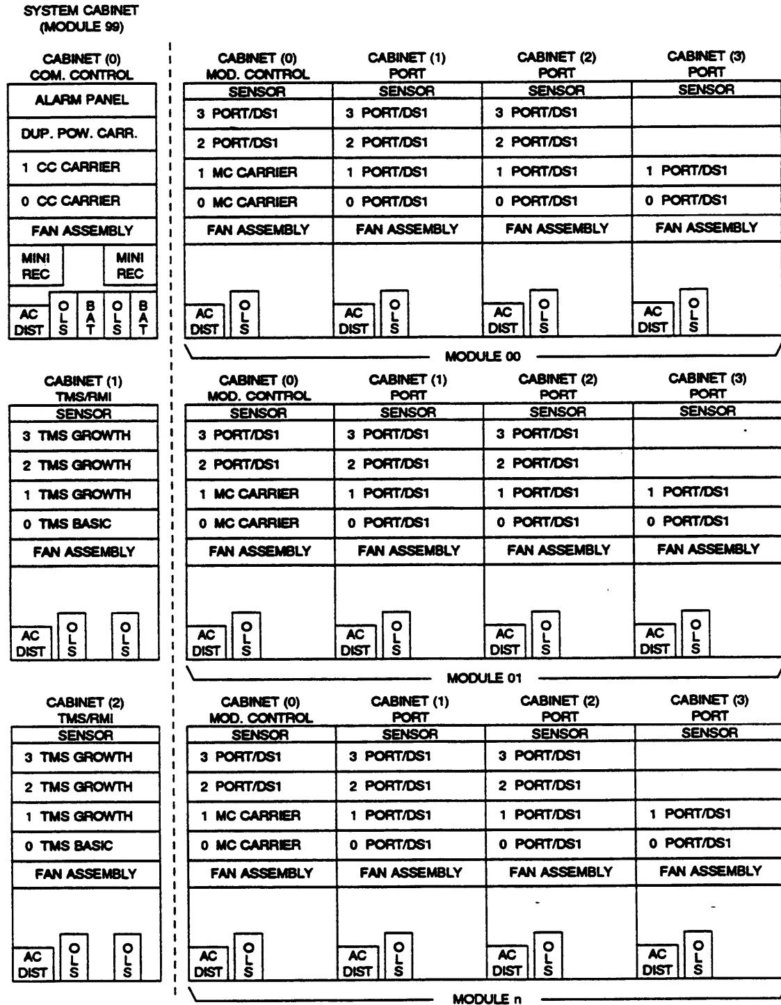
Figure 3-24. Typical Module/Cabinet/Carrier Layout for Critical Reliability Configuration
