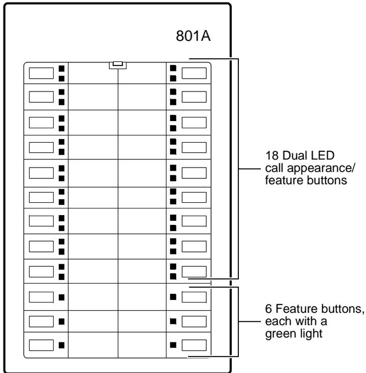
**Figure 20-4. The 801A Expansion Module**
