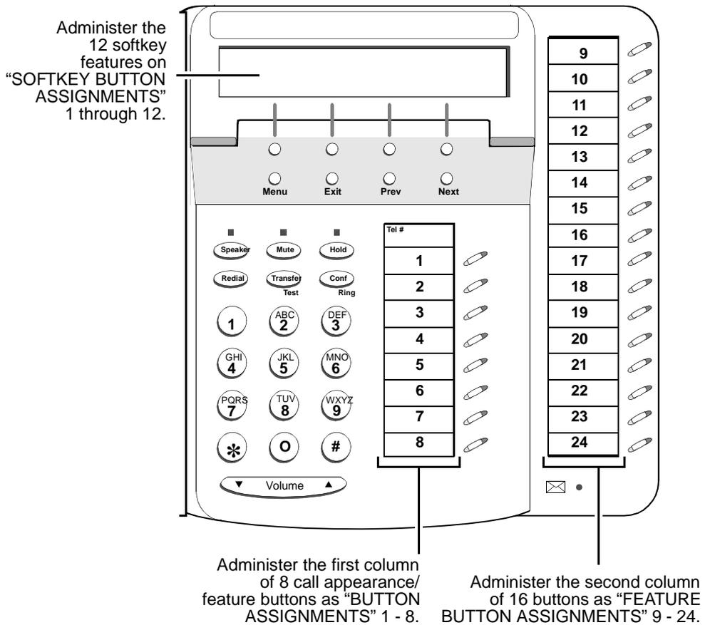
**Figure 7-10. Button Numbering for Administering the 6424D+ or 6424D+M Telephone Connected to a DEFINITY System Release 6.1 or Later**
