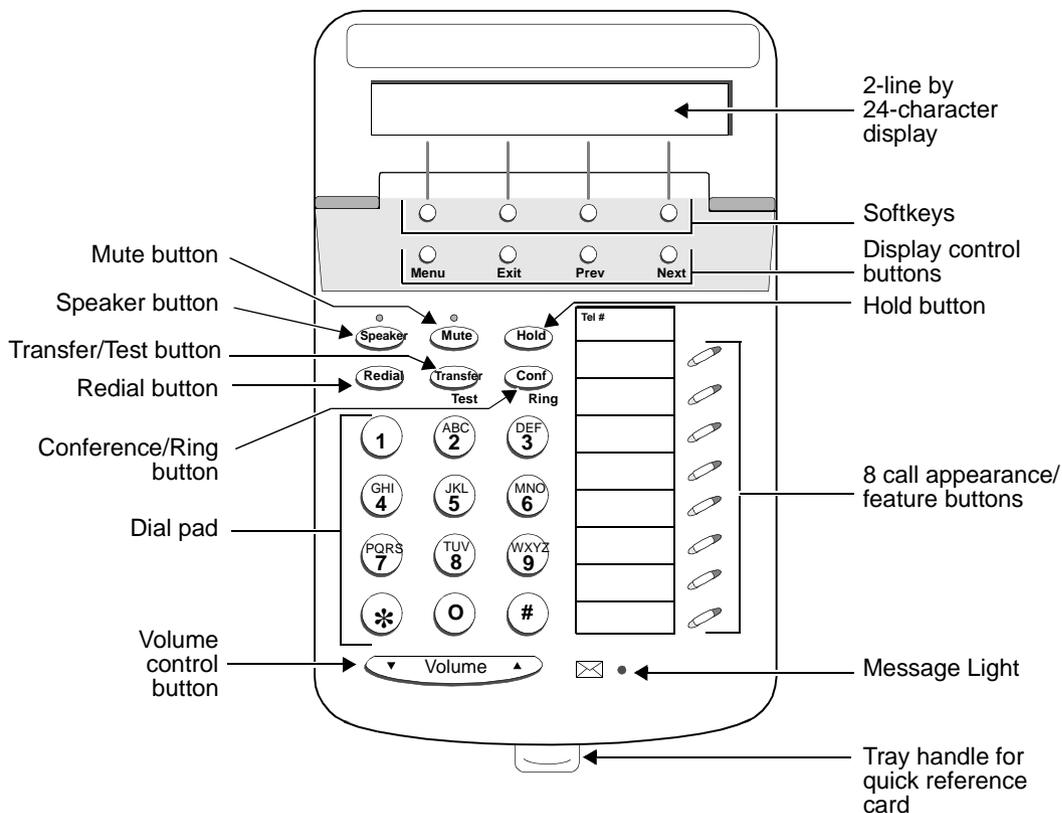
**Figure 7-5. The 6408D+ Telephone (With Display)**
