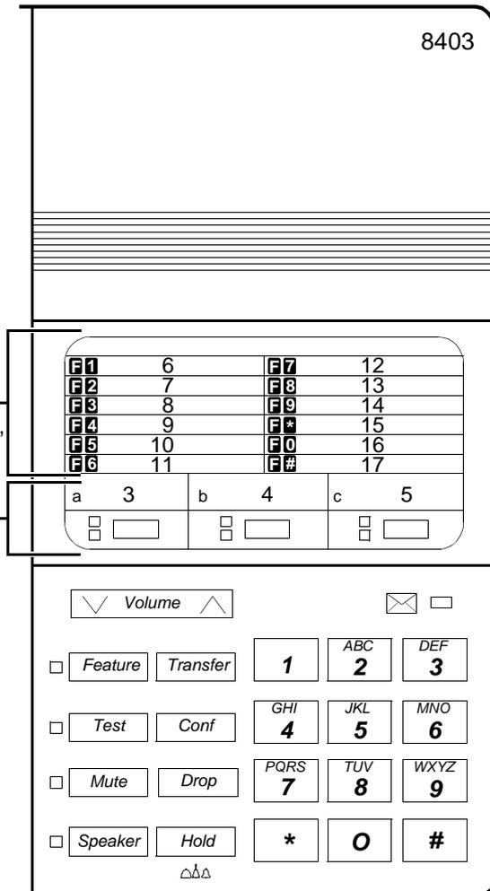
**Figure 12-4. Button Numbering for Administering the 8403 Voice Terminal Connected to a System 85 or a DEFINITY G2**
