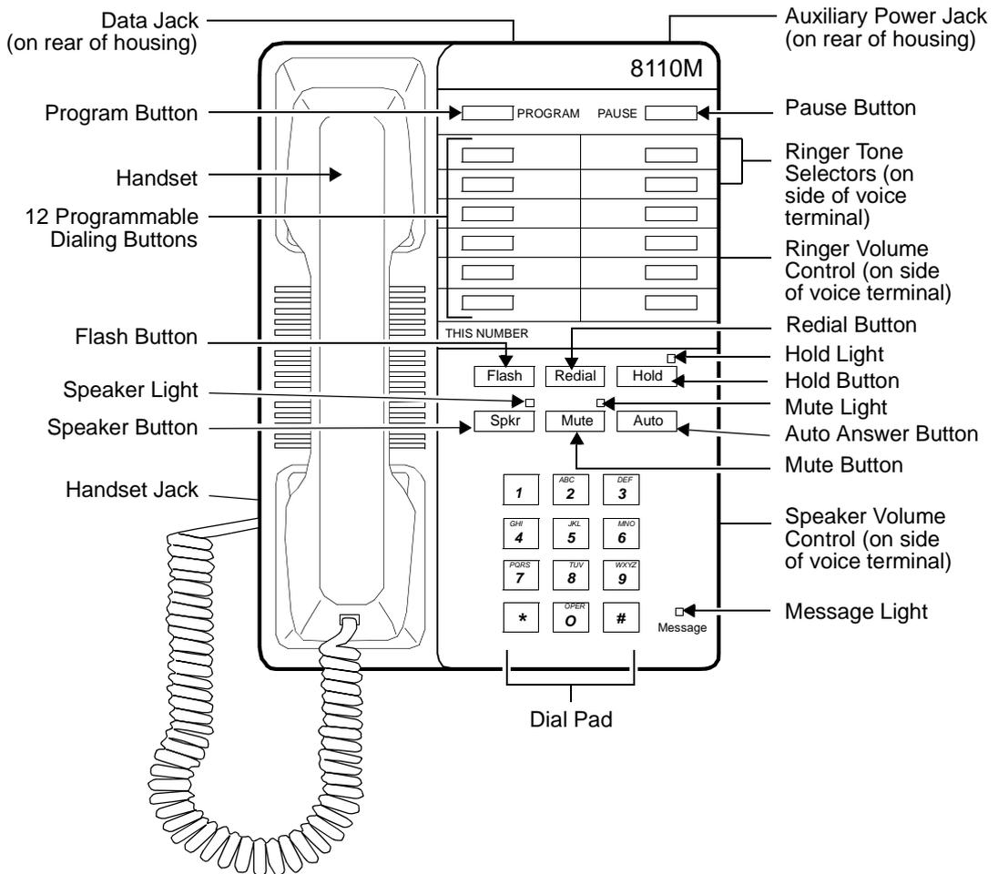
**Figure 16-4. The 8110 and 8110M Telephones (The 8110M is shown here)**
