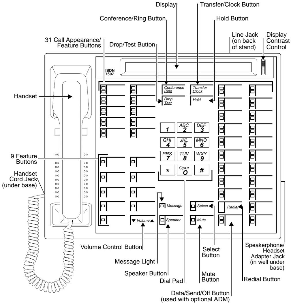
Figure 17-3. The 7507 Asynchronous Data Modular Display Terminal
