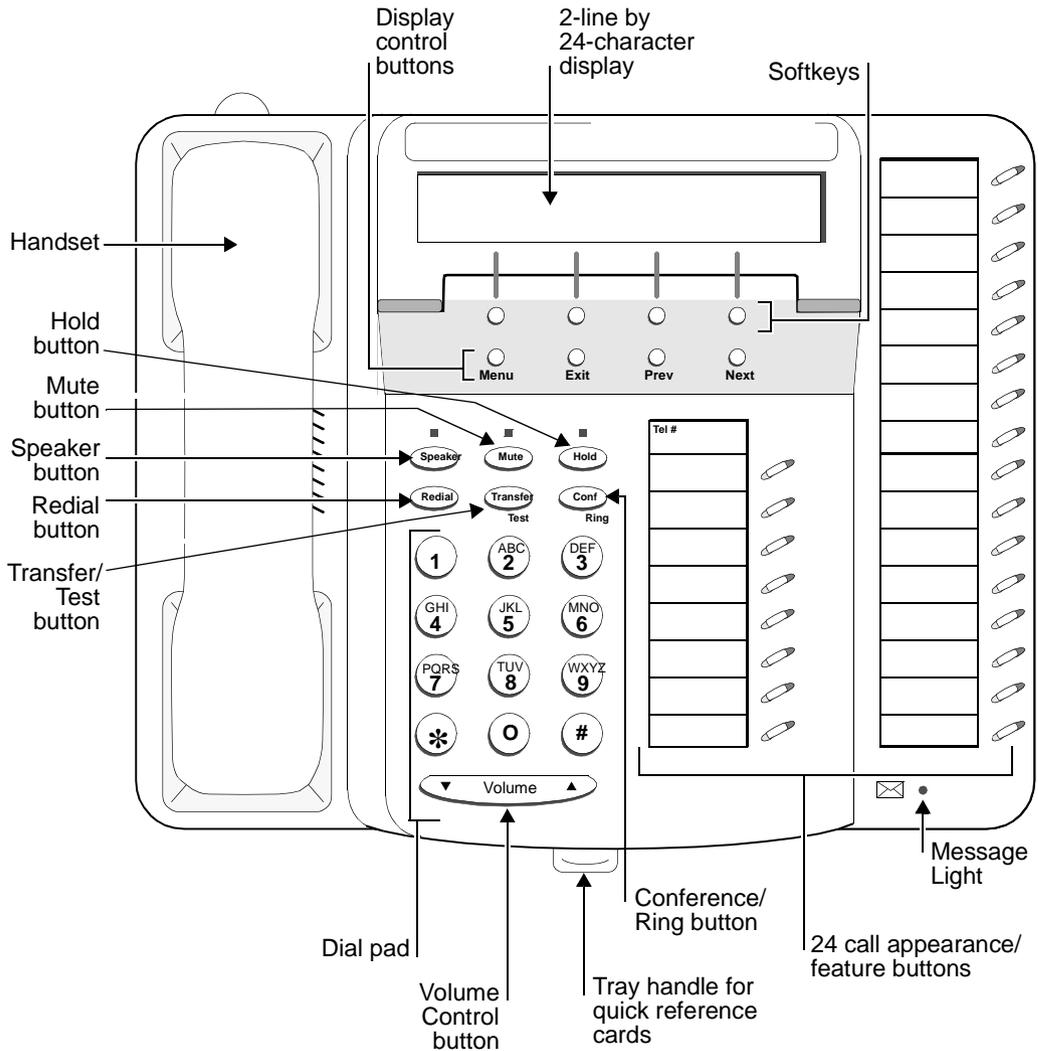
**Figure 7-9. The 6424D+ and 6424D+M Telephone**
