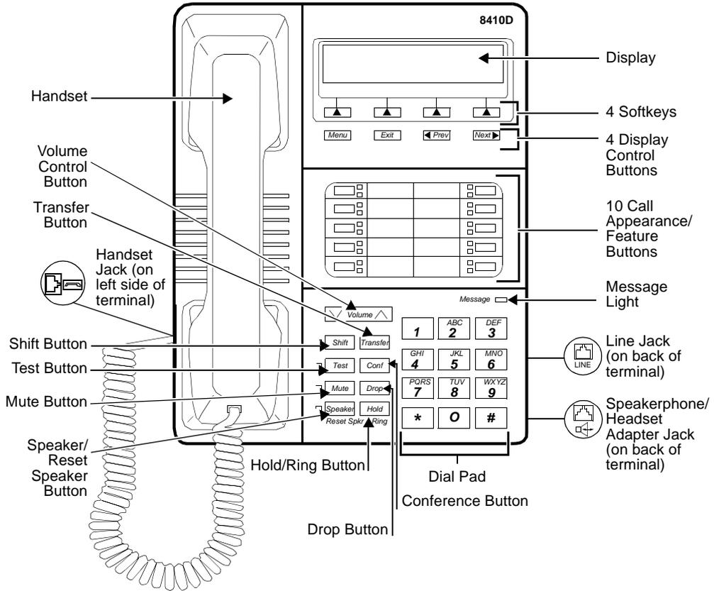
Figure 12-11. One Version of the 8410D Voice Terminal (with Display)
