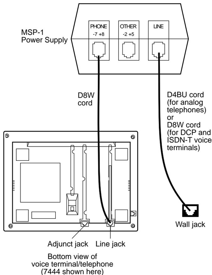
**Figure 4-2. Local Powering Arrangement (Using the MSP-1) for: ISDN-T Voice Terminals; the DCP 7444 and 8434/8434DX Voice Terminals (for their VF Displays); and Adjuncts Connected to All Telephones Except the 8102**
