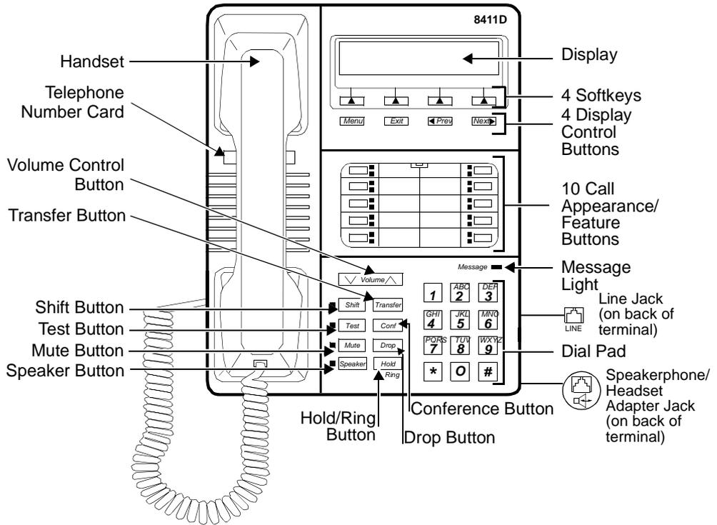
Figure 12-15. The 8411D Voice Terminal (With Display)
