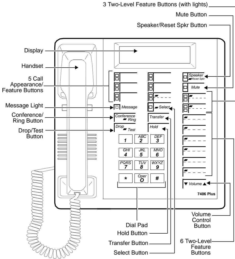
**Figure 11-12. The 7406 Plus (7406D07A) Voice Terminal with Display**
