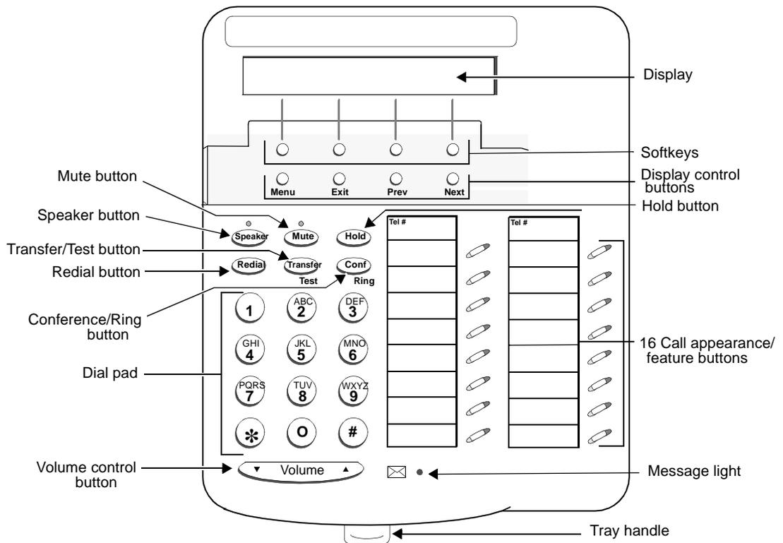
Figure 7-7. The 6416D+ and 6416D+M Telephone
