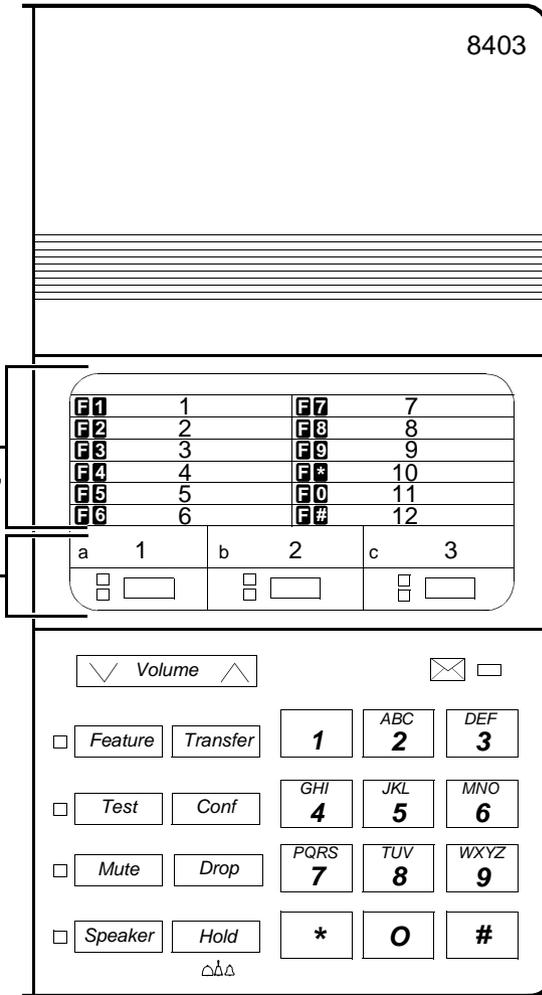
**Figure 12-3. Button Numbering for Administering the 8403 Voice Terminal Connected to a System 75, DEFINITY G1 or G3, or DEFINITY ECS**
