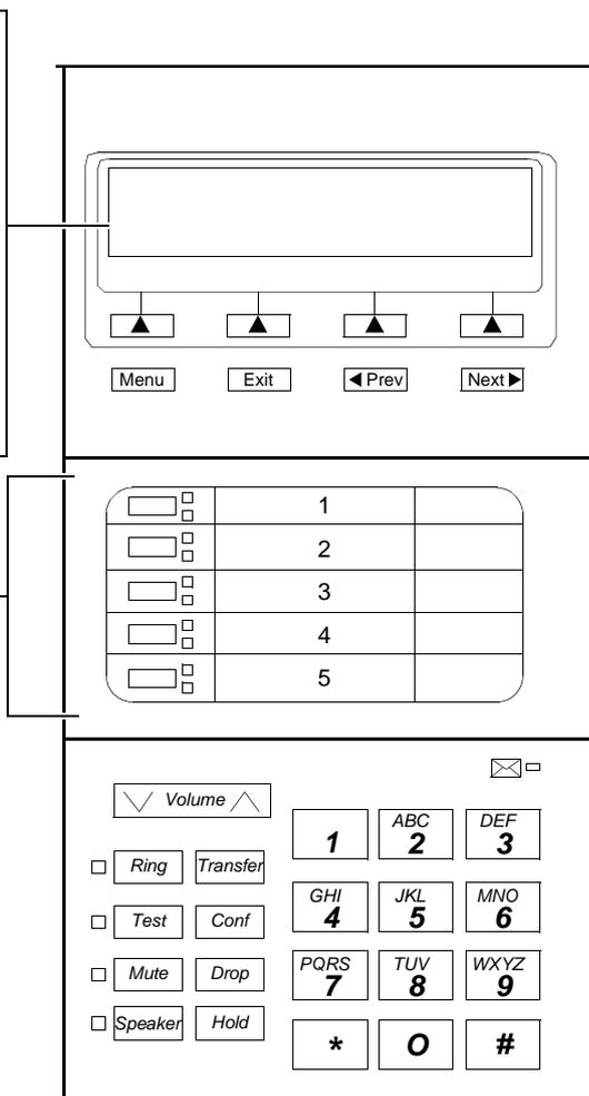
**Figure 12-9. Button Numbering for Administering the 8405 Voice Terminal Connected to a System 75, a DEFINITY G1 or G3, or a DEFINITY ECS**
