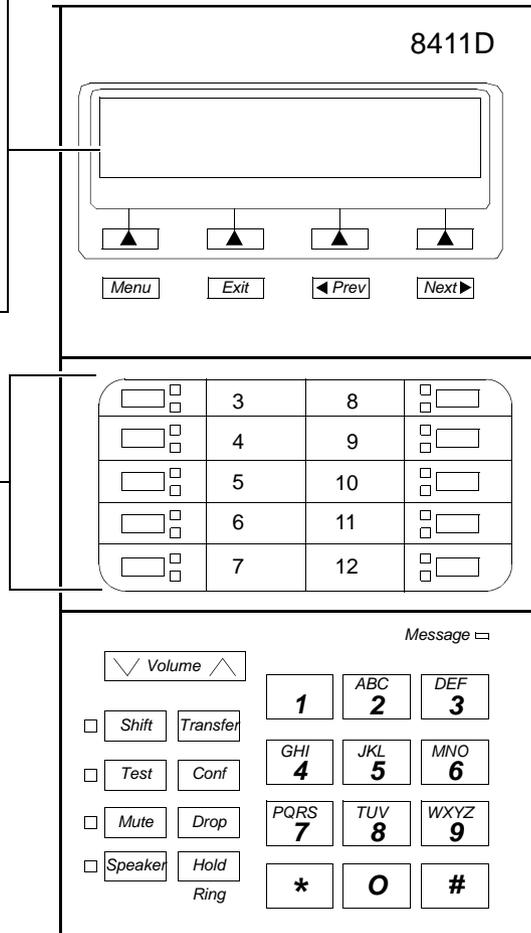
**Figure 12-19. Button Numbering for Administering the 8411 Voice Terminal Connected to a System 85 or a DEFINITY G2**
