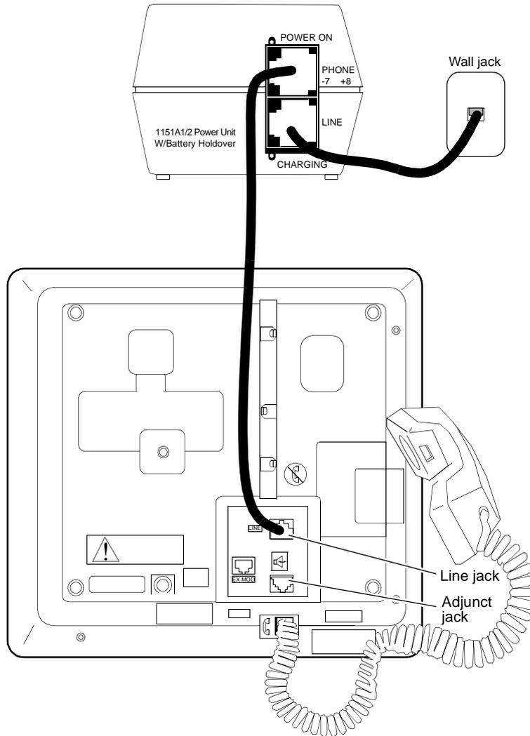
**Figure 4-4. Local Powering Arrangement (Using the 1151A1/A2) for: ISDN-T Voice Terminals; the DCP 7444 and 8434/8434DX Voice Terminals (for their VF Displays); the 8411; any 8400 or 6400 Series Telephone with an Attached Expansion Module; and Adjuncts Connected to All Telephones Except the 8102**
