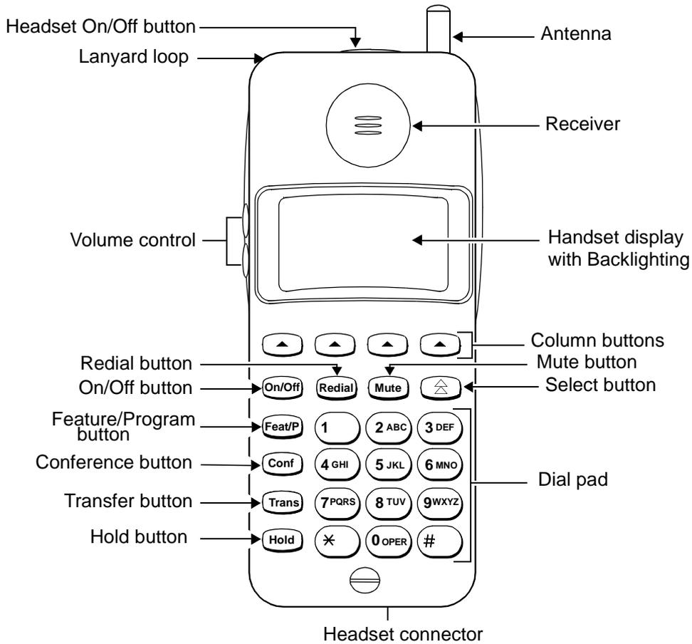
Figure 18-10. The MDW 9031DCP Wireless Pocket Phone
