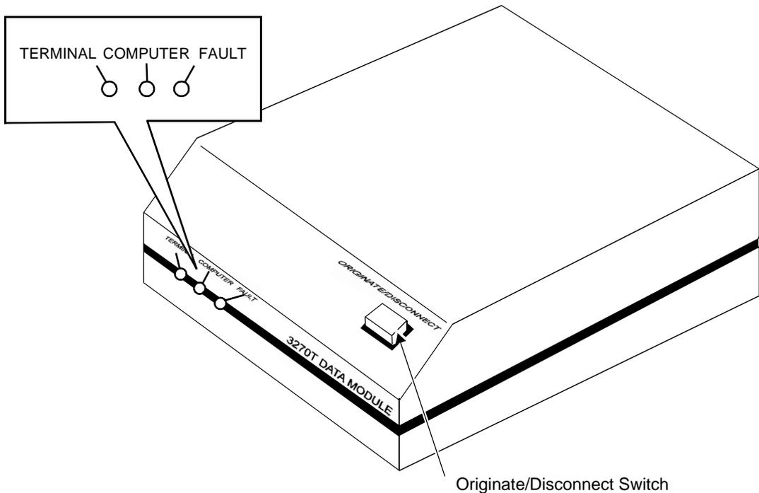
**Figure 21-23. The 3270A or 3270T Data Module**
