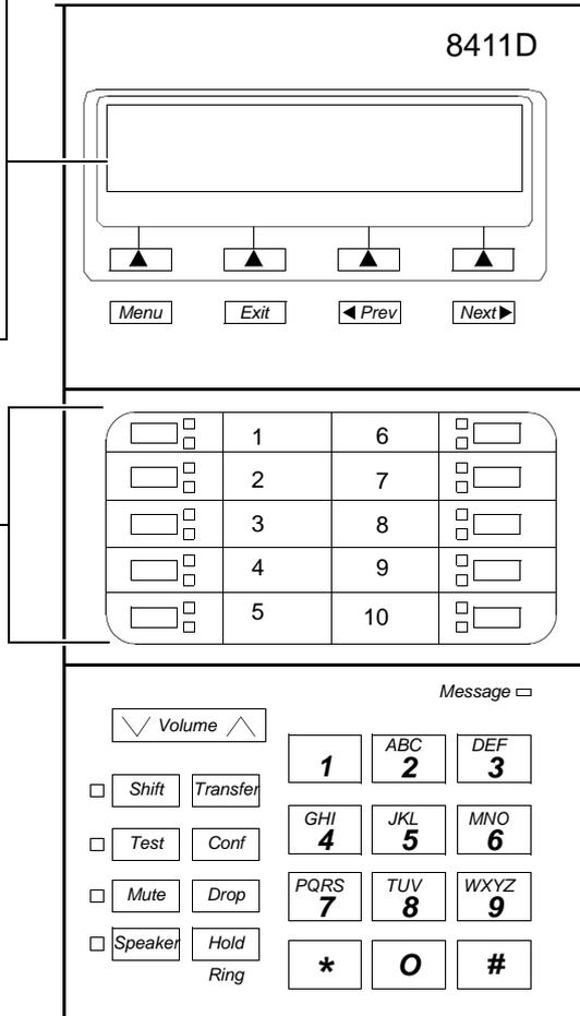
**Figure 12-18. Button Numbering for Administering the 8411 Voice Terminal Connected to a System 75, a DEFINITY G1 or G3, or a DEFINITY ECS**
