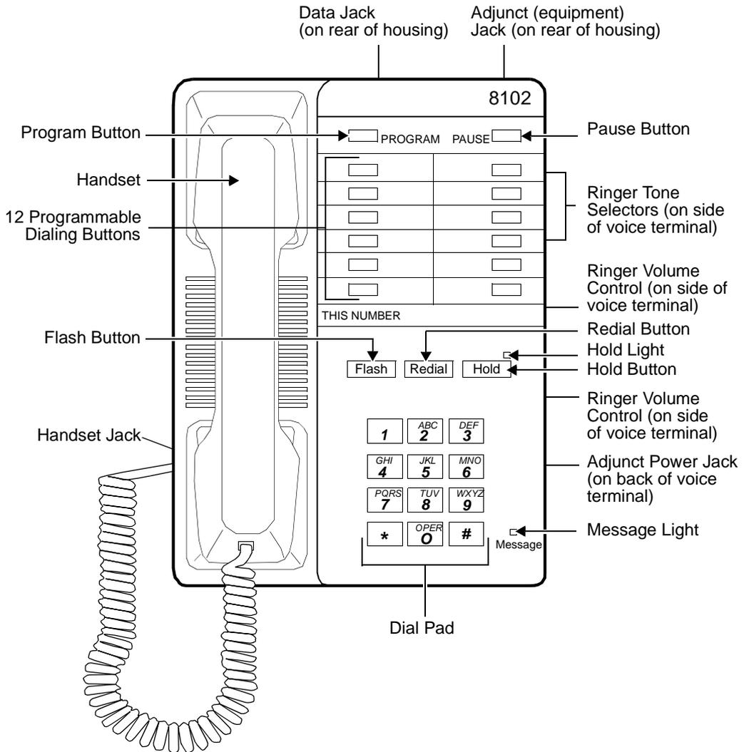
**Figure 16-3. The 8102 and 8102M Telephone**
