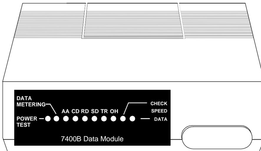
**Figure 21-2. The 7400B Plus Data Module**
