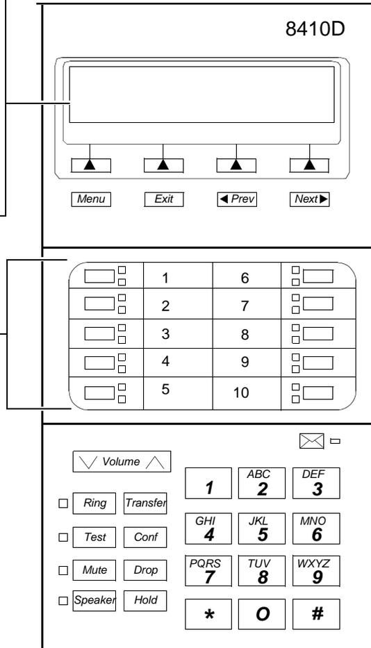
**Figure 12-13. Button Numbering for Administering the 8410 Voice Terminal Connected to a System 75, a DEFINITY G1 or G3, or a DEFINITY ECS**
