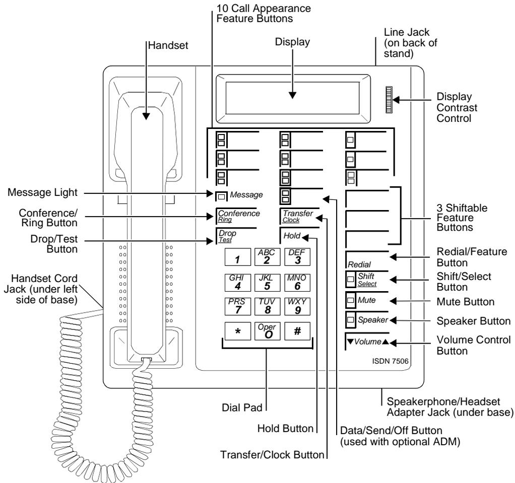
**Figure 17-2. The 7506 Asynchronous Data Modular Display Terminal**
