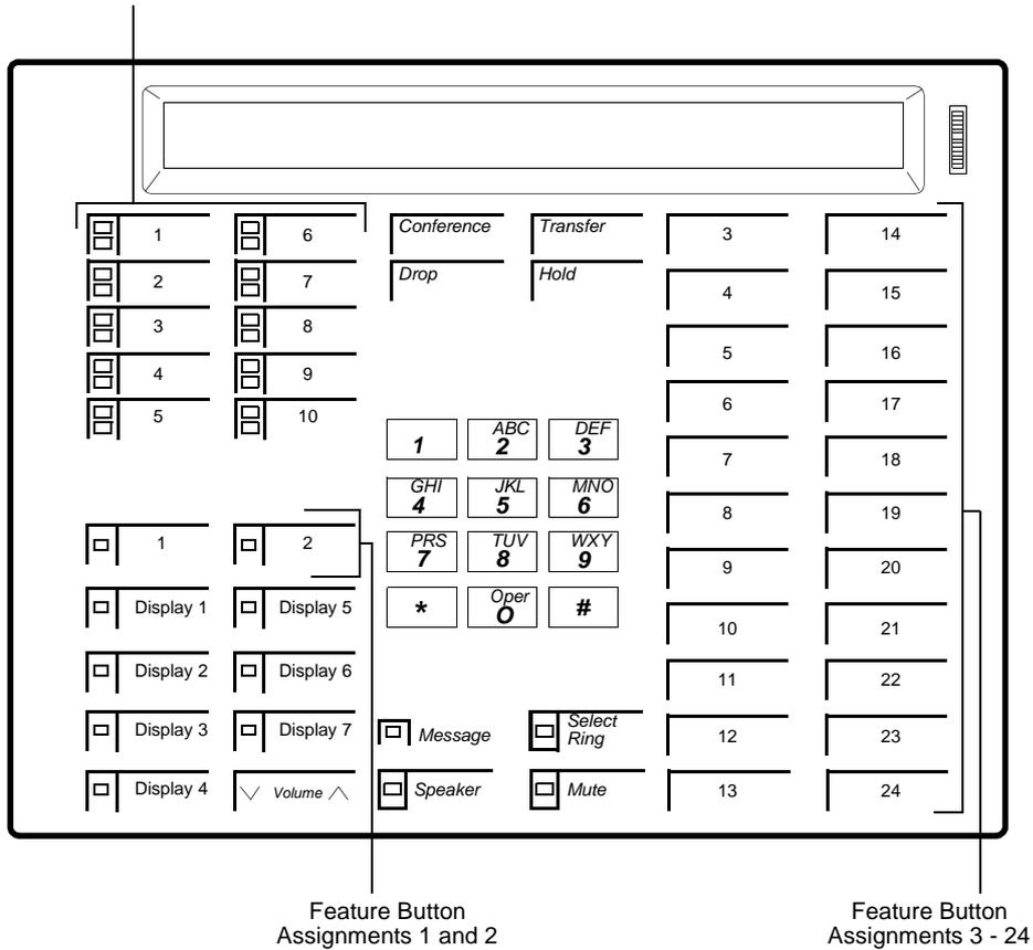
**Figure 11-22. Button Numbering for Administering the Enhanced 7407D (7407D02C) Voice Terminal Connected to a System 75, a DEFINITY G1 or G3, or a DEFINITY ECS**
