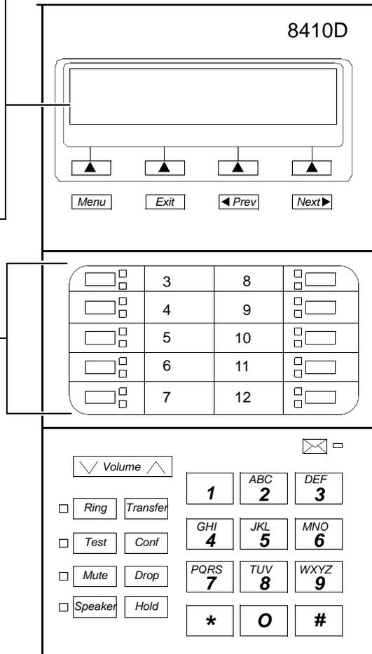
**Figure 12-14. Button Numbering for Administering the 8410 Voice Terminal Connected to a System 85 or a DEFINITY G2**
