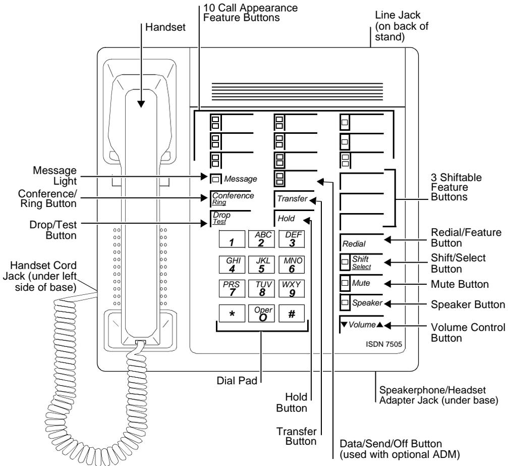
Figure 17-1. The 7505 Asynchronous Data Modular Terminal
