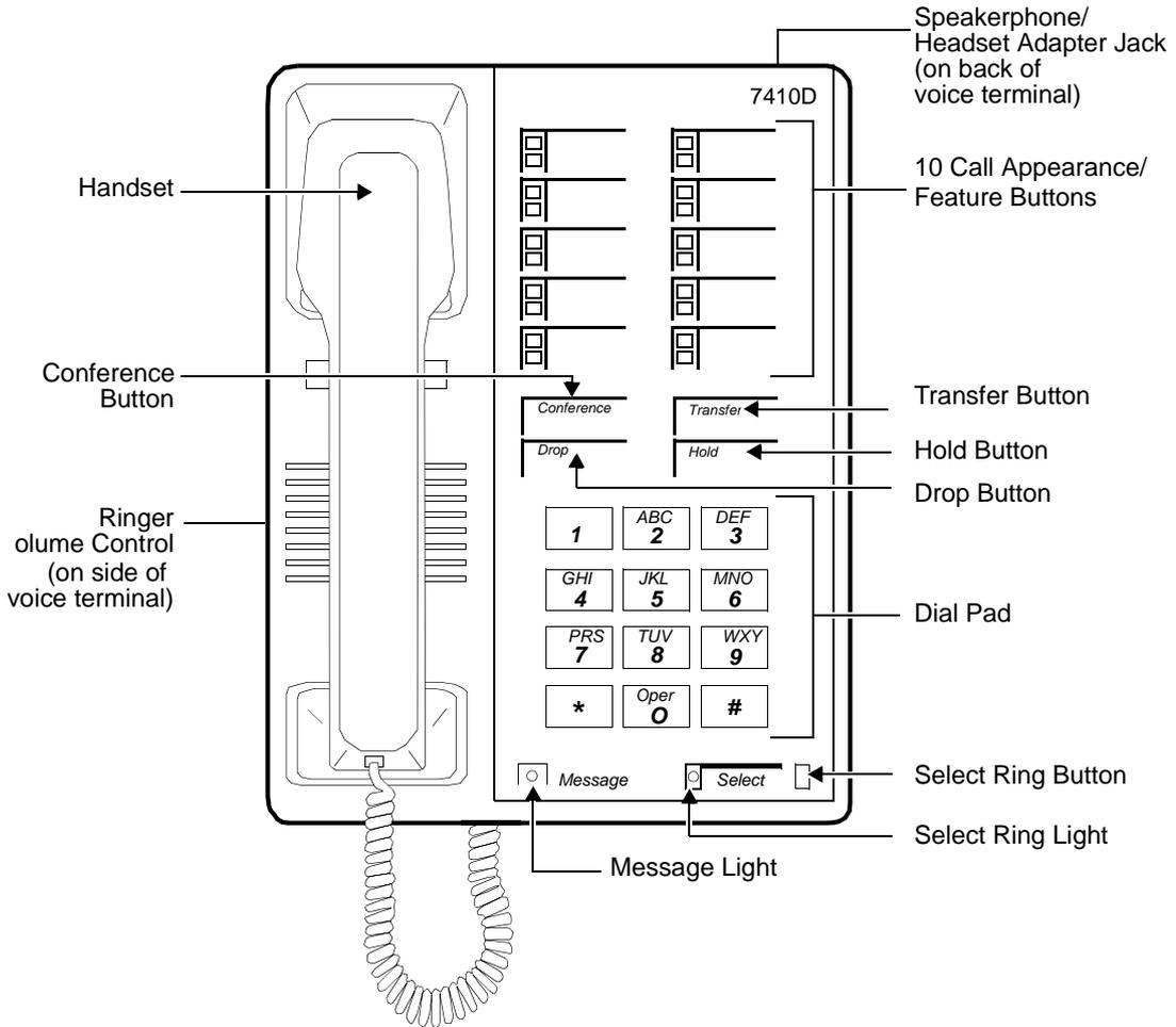
Figure 11-26. The 7410D (7401D01A) Voice Terminal
