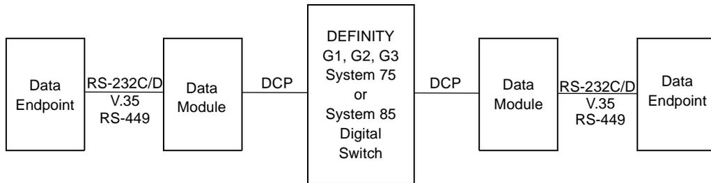
**Figure 2-3. Data Link Components**
