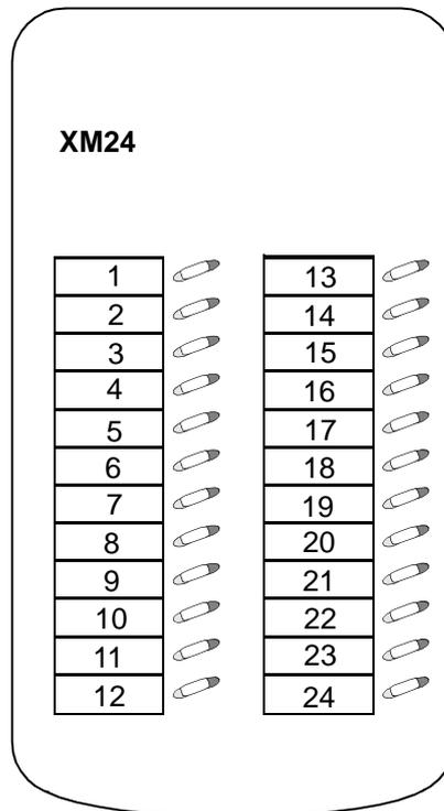
**Figure 20-7. Button Numbering for Administering the XM24 Expansion Module**
