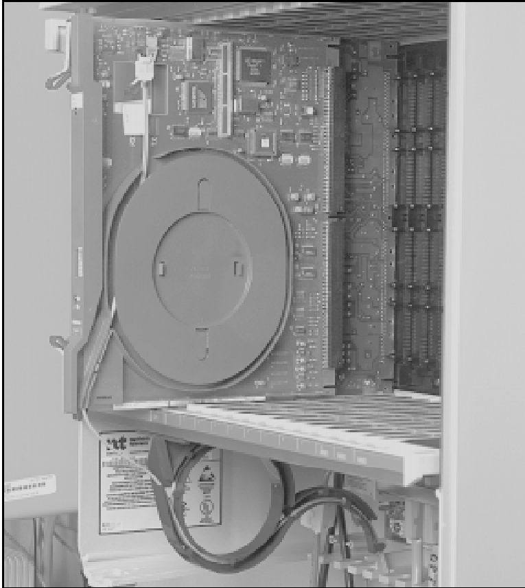
Figure 13 Fiber Receiver card for expansion cabinet (NTDK23 shown)
