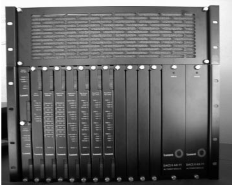
Figure 10-1. N+1 Protection Switch and DACS II AX 11
