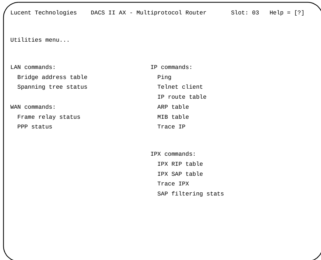
Figure 20-67. Router Utilities Menu
