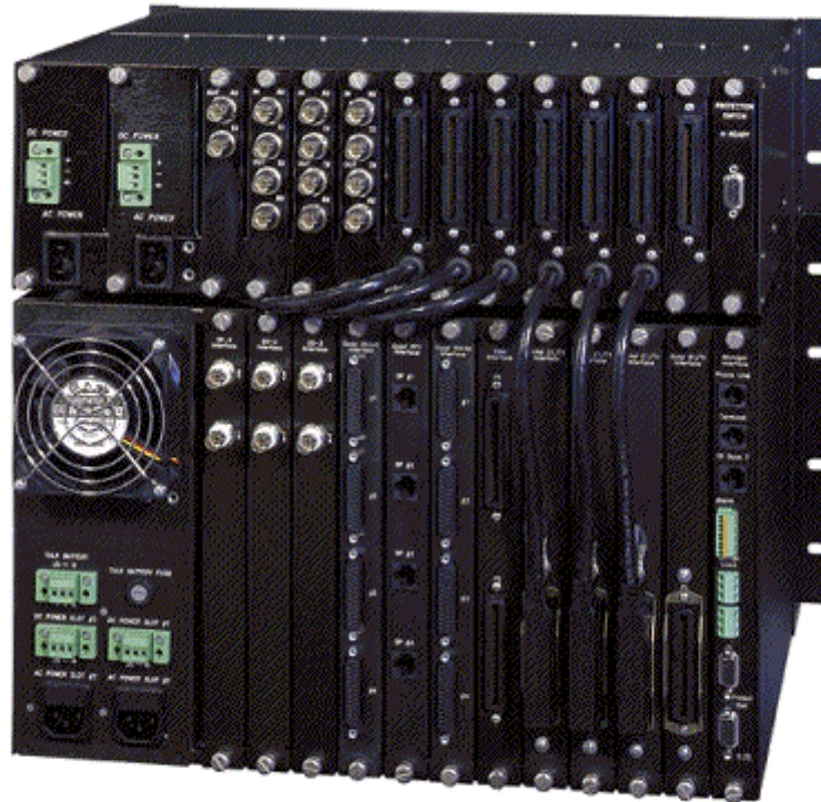
Figure 10-2. N+1 Protection Switch and DACS II AX 11 (rear view)
