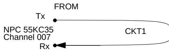
Figure G-6. Sample Half-Duplex Loopback Circuit
