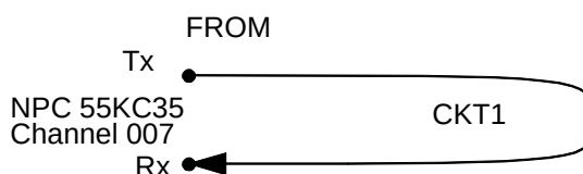
Figure 9-6. Sample Half-Duplex Loopback Circuit
