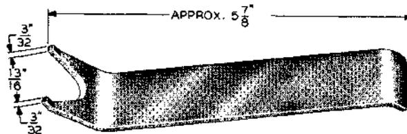
For use on compressor-dehydrators, dehydrators and air dryers.
