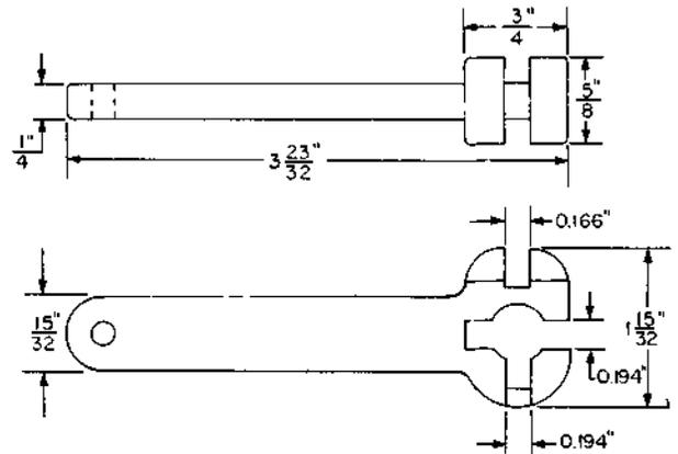
Wiper-shaft aligning wrench
