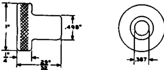
For use with the D-97083 reamer for reaming bearings in worm case housings of friction roll drives.
