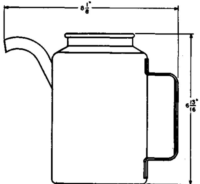
For use in filling KS-16297L1 Flushing Unit with fluid for cleaning and treating bank contacts of Step-by-Step switches.
