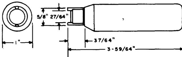
Replaces the 82 tool. For use on 223-type keys.
