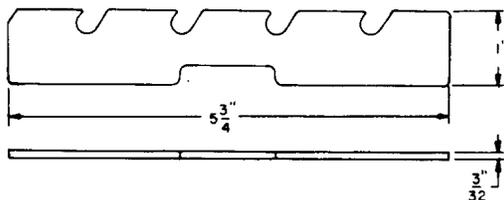
Spring support. Replaces the 543A tool. For use on 245-, 254-, 263-, and 264-type relays.
