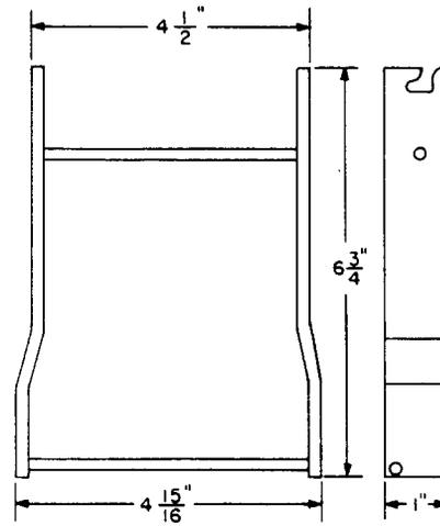
For use on step-by-step type relays and 197- and 198-type switches.
