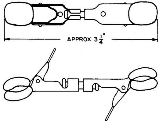
Cord support. This tool forms part of the J94724 contact closure test set. For use with the 587A tool.
