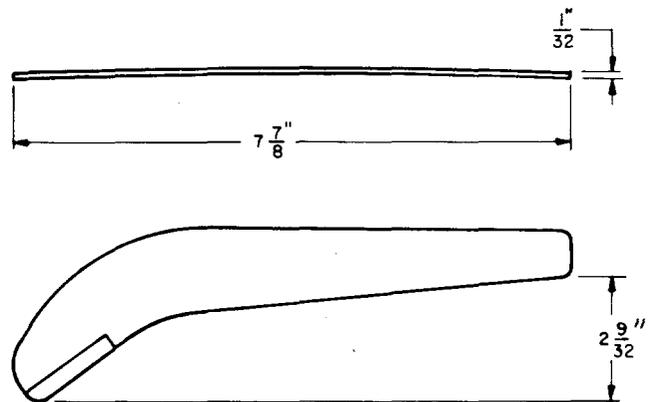
Bank contact separator. For use in cleaning plunger-type line switch banks.
