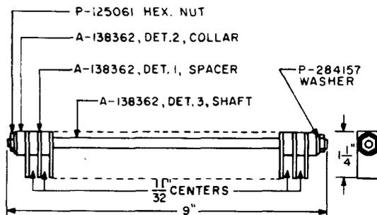
Spring separator. For use on A- and B-type sequence switches.
