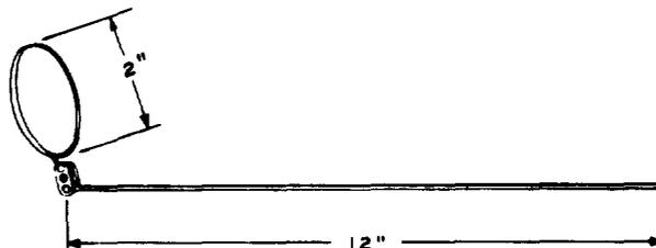
A plain adjustable mirror. For use in adjusting the KS-13834 perforators in the No. 5 Crossbar System.
