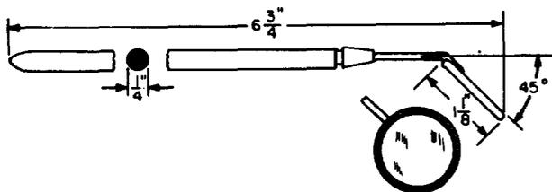
A magnifying dental mirror with the metal surfaces insulated. Replaces the R-1623 dental mirror. For use on elevator apparatus, relays, 200- and 206-type selectors, and 197- and 198-type switches.
