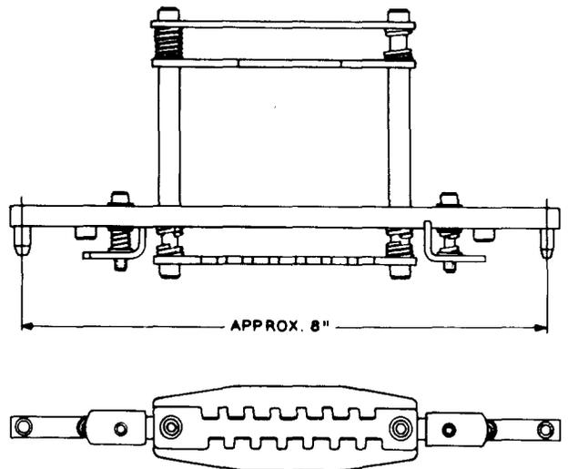
Pin locking tool. Replaces the D-178386 tool. For securing the perforator pins on a KS-13882 perforator during shipment in the KS-14131 carrying case.
