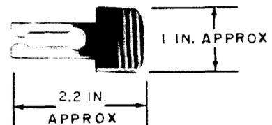
Locking tool. To lock the horizontal select bar on CA through CF types of small crossbar switches.
