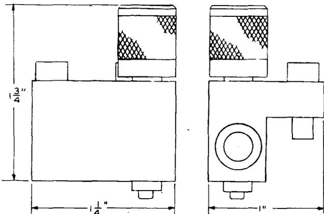
Dial locking tool. Replaces the D-178352 tool. For use as a dial lock on the KS-13835 readers in AMA Systems while adjustments are being made.
