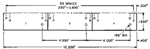
Locating and identifying tool. Used to locate and identify terminals for purposes of wiring and testing during manufacturing, installation, and maintenance. Initial use is on No. 1 ESS, J1H012A, and J1H013A switch units.
