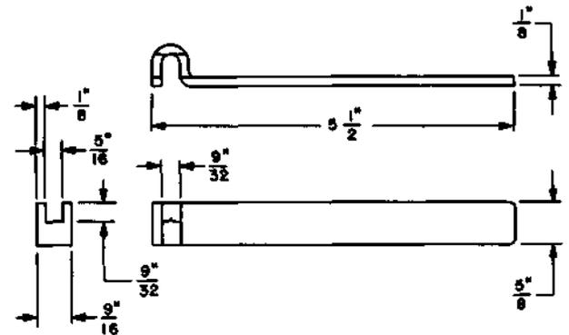
Guide holder. For use in adjusting 1-type guides.
