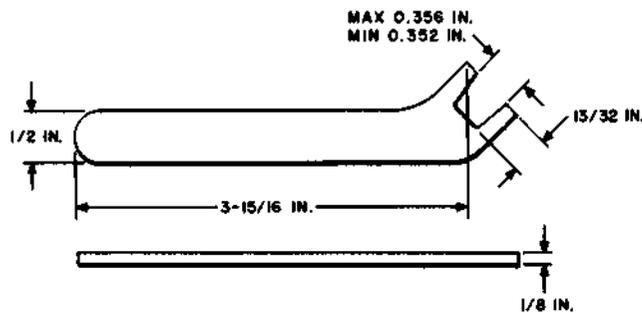
Selecting bar holder. Replaces the 536A tool. For use on 300-, 304-, 314-, 324-, and similar-type switches.
