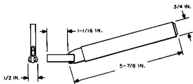
Relay core holder. For use on U-, UA-, and Y-type relays having hinge pin-type armature suspension.
