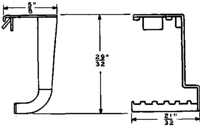
Spring holder. For use in holding the lower group of movable break contact springs on AF-, AG- and AJ-type relays during removal of the card from the relay.
