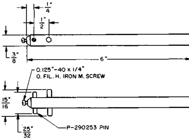
Index wheel holder. For use on A- and B-type sequence switches and 155A and 157-type interrupters.
