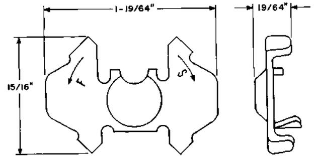
Dial governor holder. For use in holding rotating parts of 2-, 4-, and 5-type dial governors stationary when adjusting them for speed.
