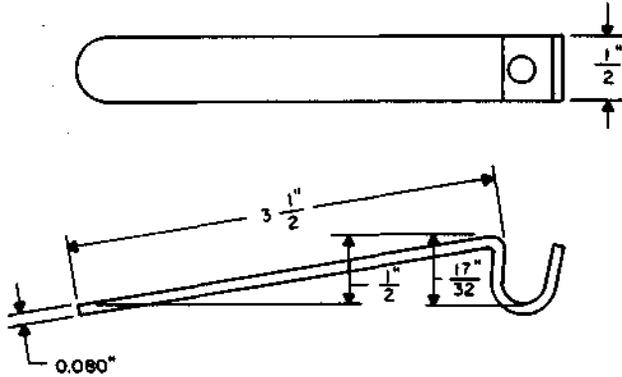
Trip rod holder. For use on 4- and 14-type trip rods.
