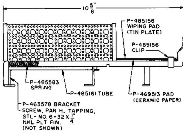
Soldering copper holder. Designed to clamp on rolling ladder steps. May also be used with ED-92008-01 mounting bracket or on a flat surface. See the 721A tool for adapter which may be added to this tool for holding KS-14440 and KS-16346 soldering coppers. This adapter cannot be used with KS-8740 soldering copper. Also see Rest, Copper, Soldering, Section 074-253-130. For general use.
