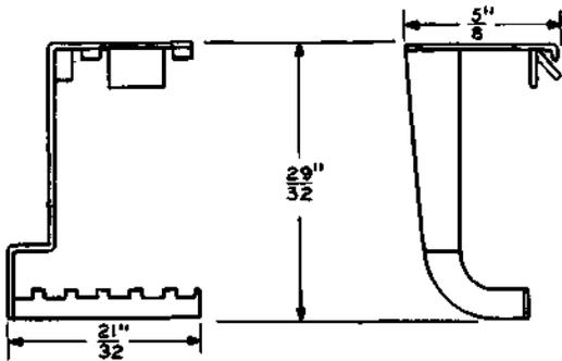
Spring holder. For use in holding the upper group of movable break contact springs on AF-, AG- and AJ-type relays during removal of the card from the relay.
