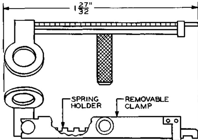
Spring holder and removable clamp. For use in holding movable make contact springs in positions 1 through 12 on AF-, AG-, and AJ-type relays during removal of the card from the relay.
