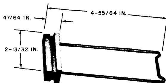
Ratchet head. This tool forms part of 1014B tool kit. For use in conjunction with 715A tool when replacing coils of AF-, AG-, and AJ-type relays.
