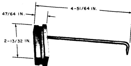
Ratchet head. This tool forms part of 1014B tool kit. For use in conjunction with 715A tool when replacing coils of AK-type relays.
