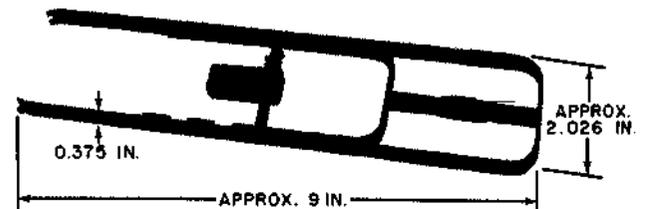
Circuit pack extractor. For use in extracting Amplas circuit packages from frame mounted KS-19437 connectors in common systems.
