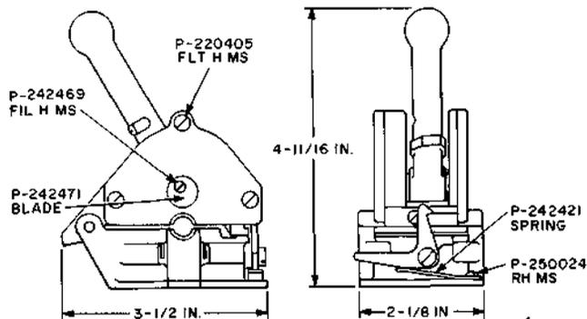
Cord cutter. The base is provided with screw holes for attaching to the KS-5263 cord repair table. For use in repairing switchboard cords by the solderless cord-tip method.
