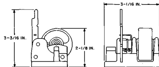
Conductor braid cutter. For use in repairing switchboard cords by the punched-hole method. The information covered herein replaces the part of Section 074-000-006, Issue 1, applying to this tool.
