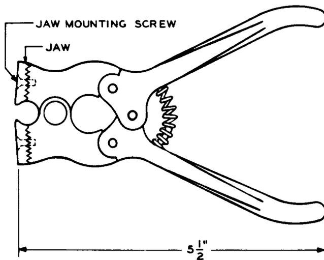
These tools are the same except for the cutting jaws. The jaws (pair) and the jaw mounting screws may be ordered separately when desired. In ordering, specify "( ) for (KS- ) cut nippers."
