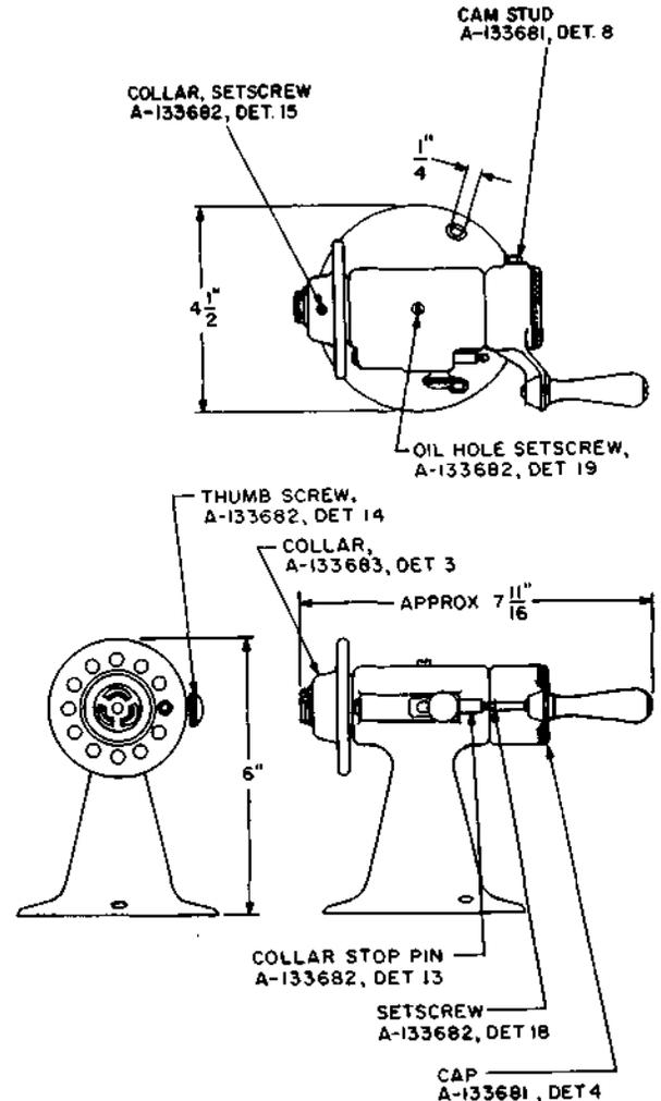
Plug removers and attachers. These tools consist essentially of a horizontal hollow shaft which is equipped with a crank and contains a chuck. This shaft is provided with a collar whereby the chuck is adjusted to grip the shoulder of a plug. The two tools are identical except for the chuck. The tools replace the 200, 201, and 202 tools.
