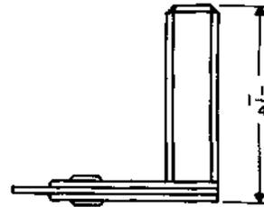
Test connector. For use in connecting to meters, etc., in checking teletypewriter equipment.
