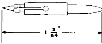
**Relay contact connector.** For use in conjunction with 360-type and 651-type tools to make test connections to the fixed contacts on AF-, AG-, AJ-, and AK-type relays.
