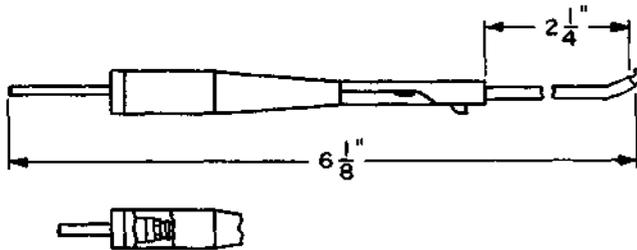
Magnet winding connector. Used in conjunction with the 360-type tool. For use on 245- and 254-type relays, 300- and similar-type switches, and 1- and 2-type timers.
