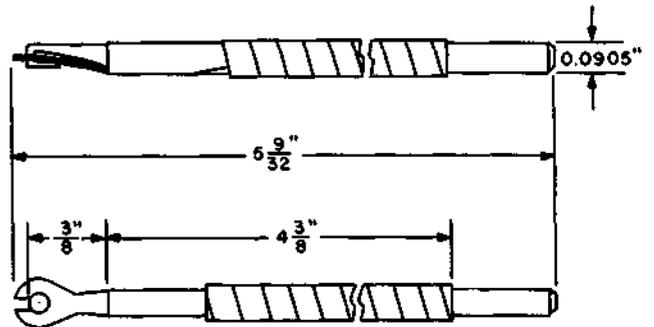
Relay winding connector. Replaces the R-2736 relay winding connector. For use on U-, Y-, and UB-type relays.
