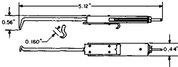
Relay winding connector. Replaces the 428A tool. For use in making test connections from the front of the relay on 89-, 101-, 105-, 108-, 111-, 121-, 122-, 149-, 162-, 172-, 178-, 179-, 190-, and 196-type relays.
