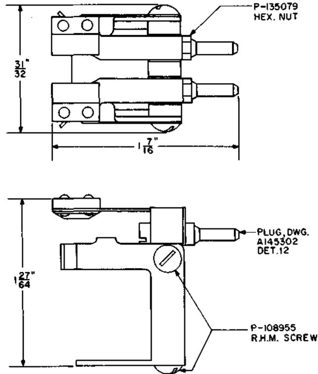
Intercontact connector. For use on 111-type relays.
