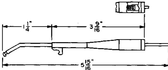
Magnet winding connector. Used in conjunction with the 360-type tool. For use on 300- and similar-type switches.
