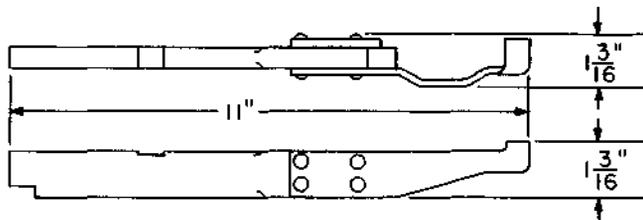
**Multiple bank carrier. For use in handling panel multiple banks. Two or more of these tools may be coupled together to obtain greater leverage.**
