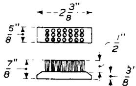
For use in cleaning protector blocks, and designed to mount on the end of the No. 3A carrying case by means of a screw which is provided.
