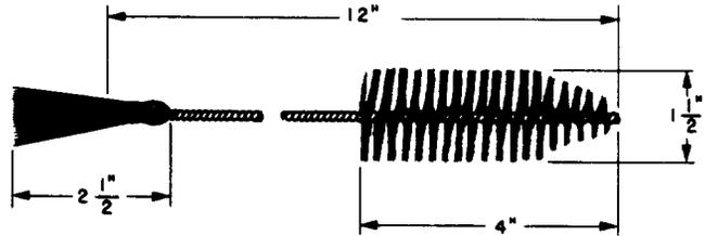
A bottle-type typewriter brush having a twisted wire handle 12 inches long. For use on friction roll drives and plunger-primary and secondary line and out-trunk switches.
