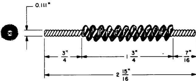
A soft nylon bristle brush. Replaces the R-2448 treating brush. For cleaning sequence switches and panel multiple banks.
