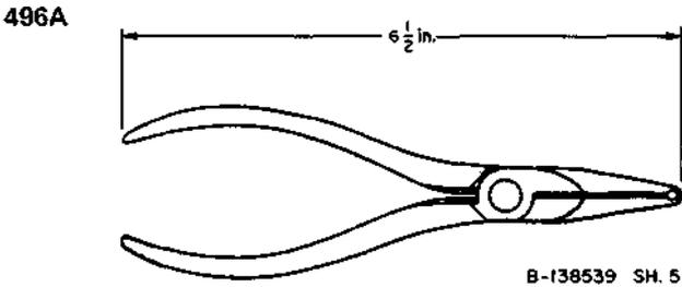
Pin Pliers. This tool forms part of the No. 1001A tool kit.
