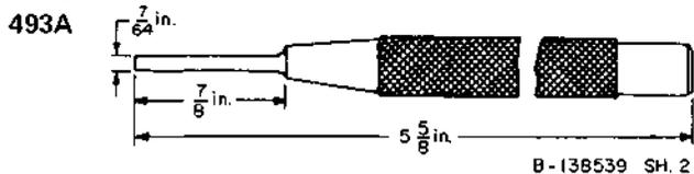
**7/64" Pin Punch.** This tool forms part of the No. 1000A tool kit. For use in replacing bushings on reciprocating bar-type interrupters.
