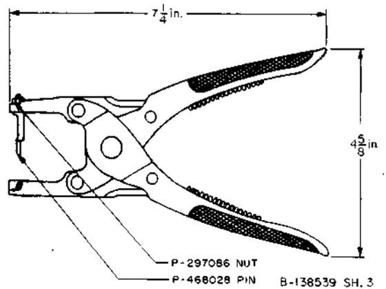
**Pawl Pin Remover.** This tool forms part of the No. 1001A tool kit.
