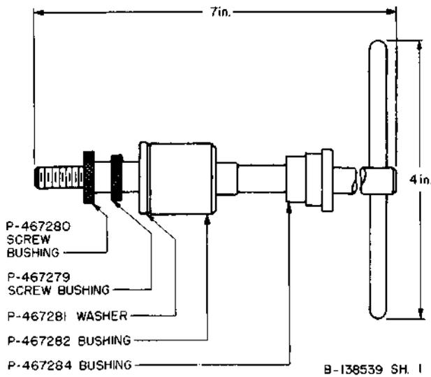
**Bushing Remover and Replacer.** This tool forms part of the No. 1000A tool kit.
