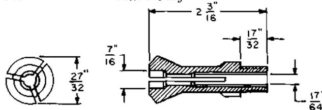
Plug remover and attacher. This tool, in conjunction with the 200 tool, is equivalent to the 317 tool. Do not order this tool unless the office is equipped with the 200 tool.
