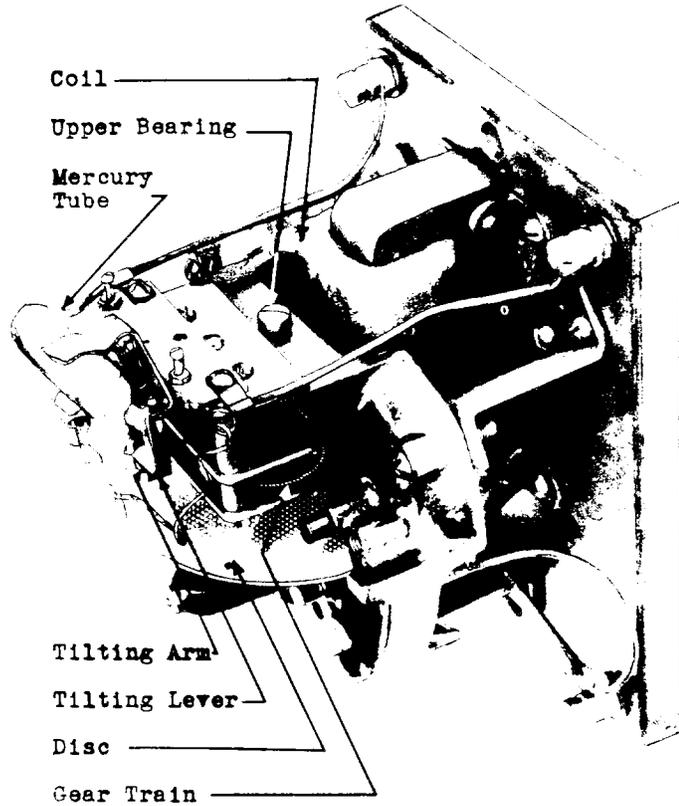
Fig. 3 - Time Delay Relay
