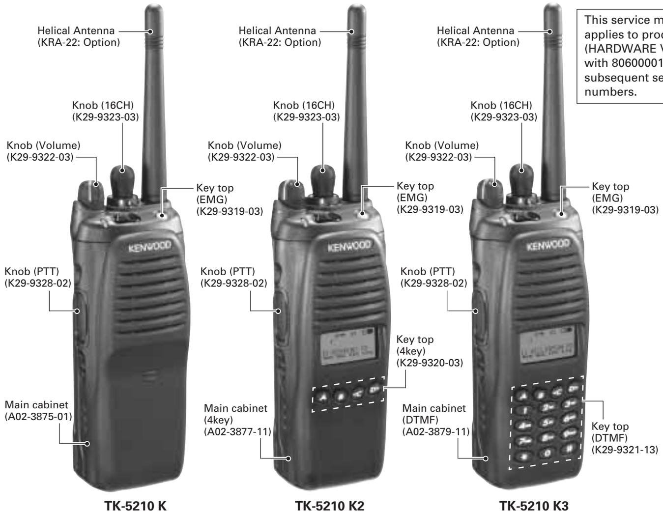
This service manual applies to products (HARDWARE VER 2.0) with 80600001 or subsequent serial numbers.
