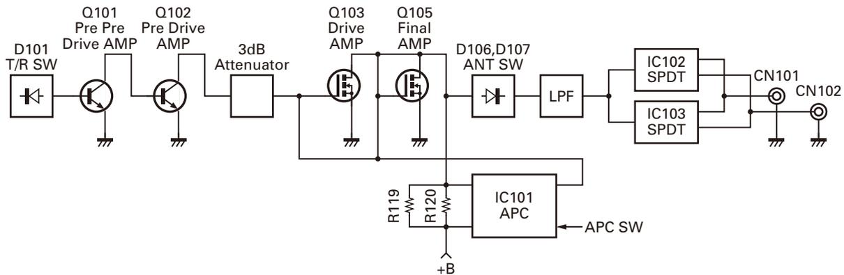
Fig. 7 Transmitter circuit
