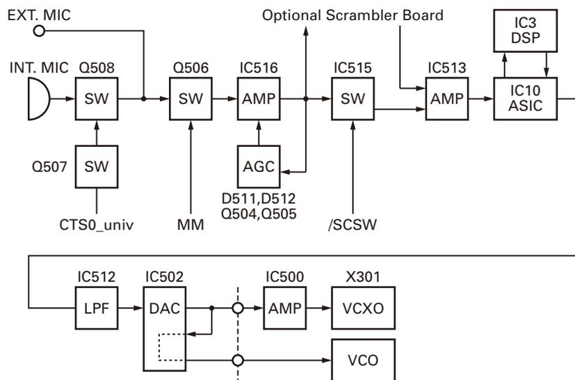
**Fig. 6 Audio band and Base band circuit**
