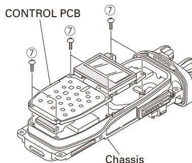
2. On the reverse side of the CONTROL PCB ⑧, remove the cord ASSY and each FPC from the connectors (CN40, CN35, CN38) of the CONTROL PCB.
