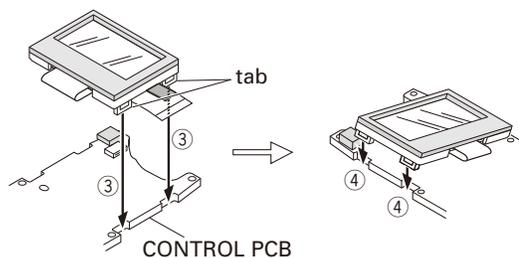
3. Insert the FPC into the CONTROL PCB connector (CN1) ⑤.
