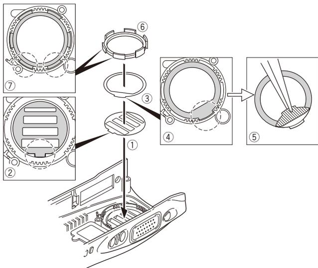
5. Verify that the packing does not ride on the rib of the case.
