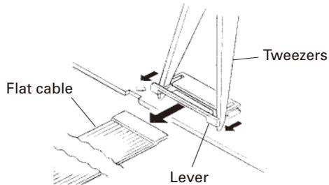
2. Gently rise up the connector lever in the direction of the arrow with a flat-head screwdriver or tweezers.
