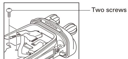
3. Firmly tighten the hexagon screws of the GND terminal.
