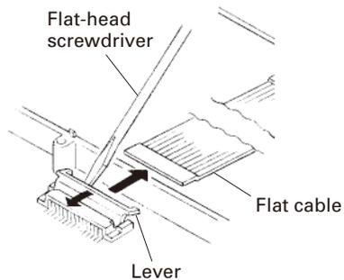
3. Gently depress the connector lever in the direction of the arrow with a flat-head screwdriver or tweezers.
