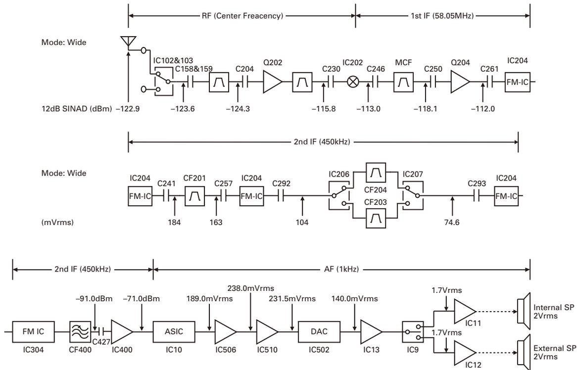
To make measurements in the AF section, connect the AC level meter.
