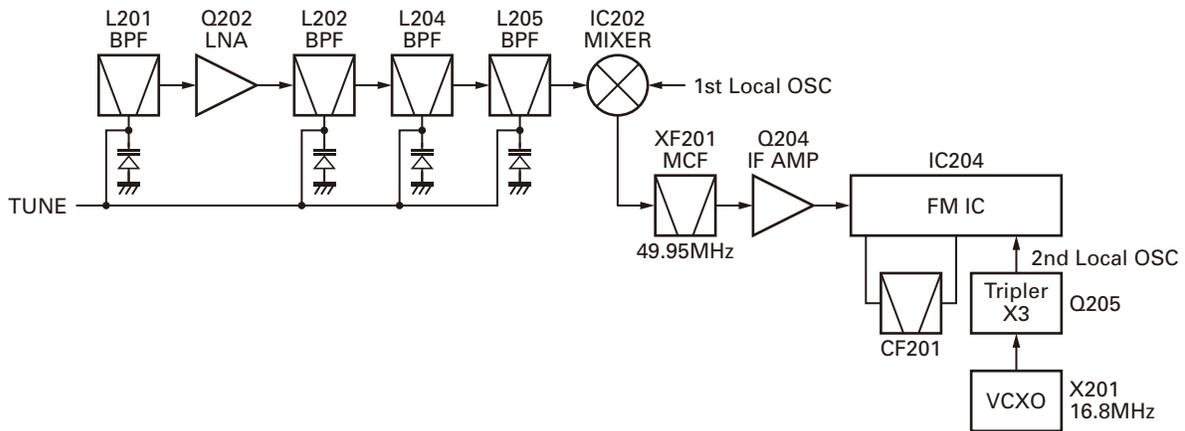
**Fig. 2 Receiver section**
