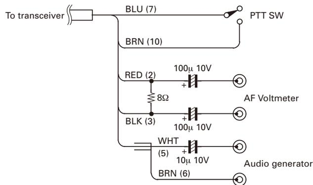
**Note:** Pin 1 (SSW) and Pin 4 (MSW) are connected to Pin 10 (GND) to active External SP and External MIC.
