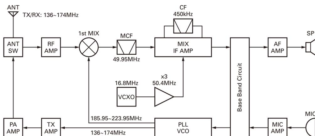
Fig. 1 Frequency configuration
