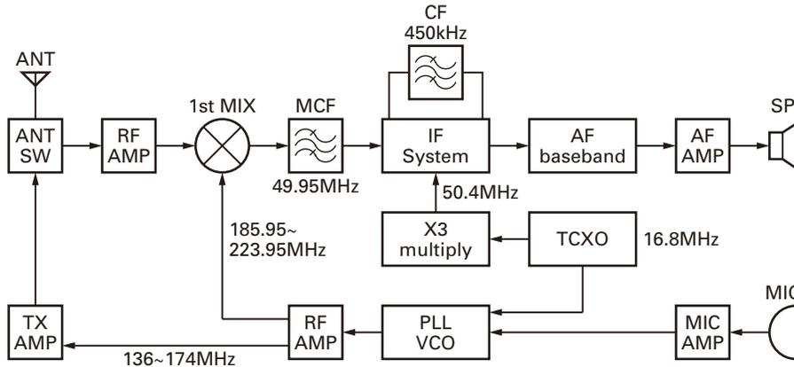
Fig. 1 Frequency configuration
