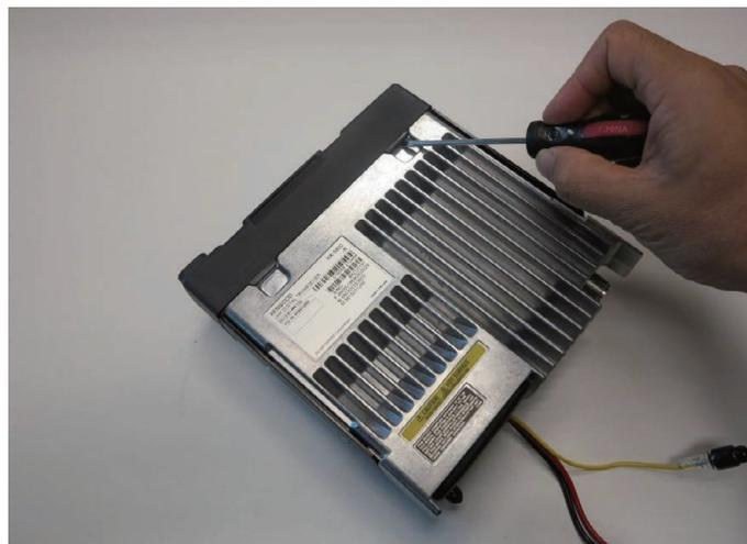
Figure 17-1 Removal of the Panel
