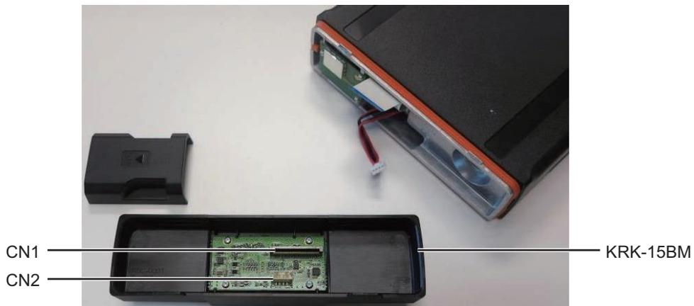
Figure 17-3 Connection of the Cables
