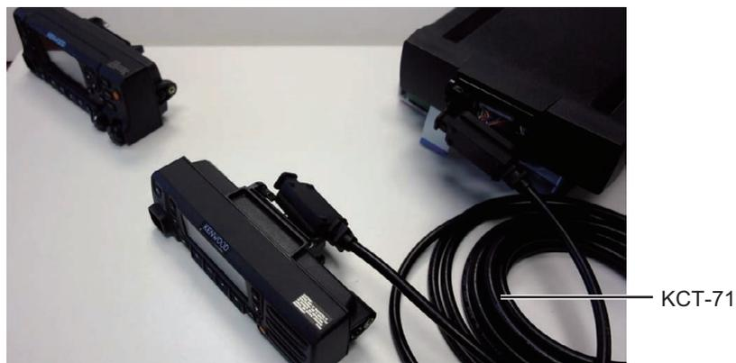
Figure 17-8 Connection of the KCT-71 Cables
