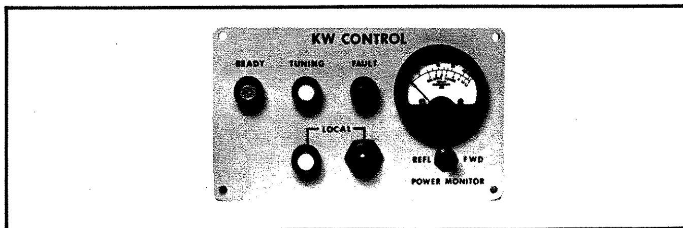
Figure 3.4 1 KW Coupler Control Panel
