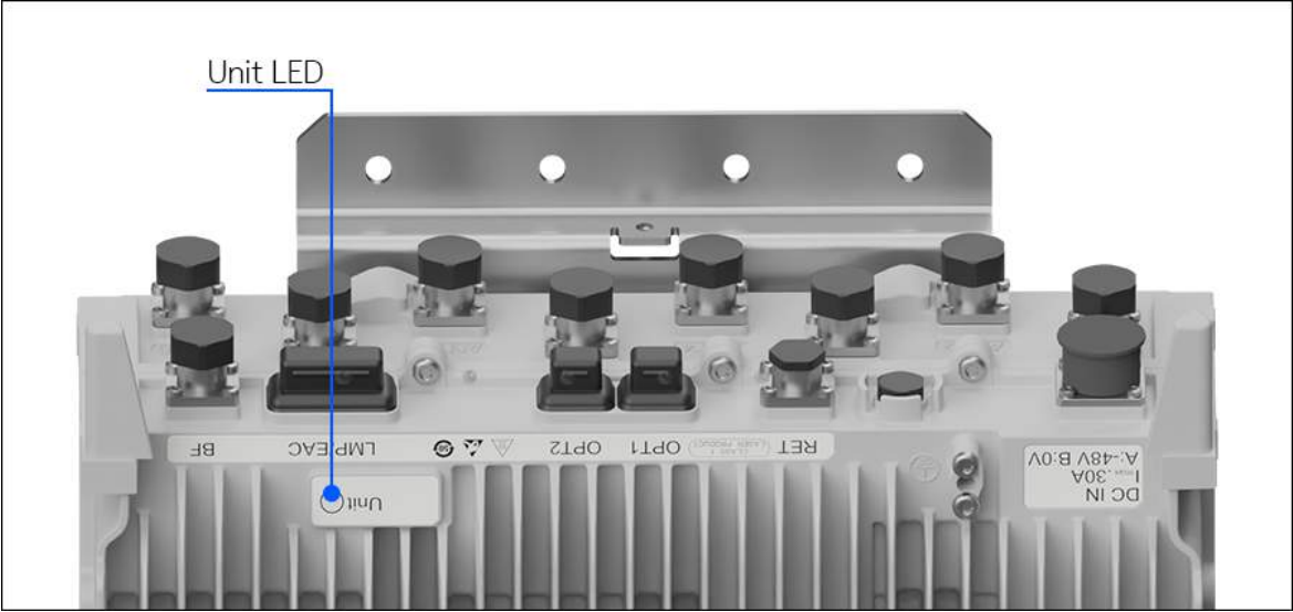
Figure 305: AirScale 2 TDD RU (2T2R/4T4R/8T8R) LED interface
