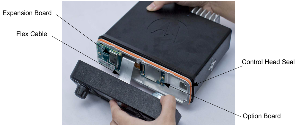
Figure 5-2 Flexible Connection Removal
