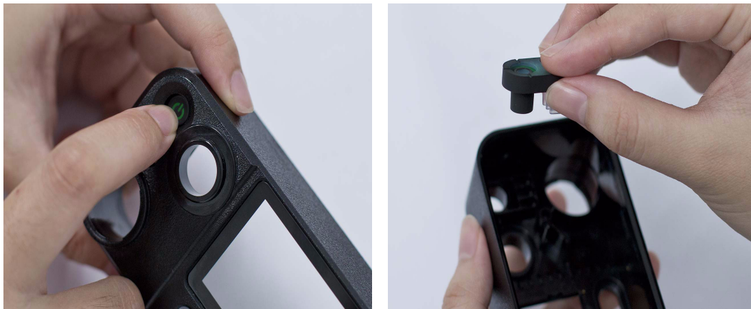
Figure 5-41 Power Button Removal
