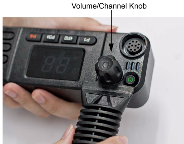
Figure 5-38 Volume/Channel Knob Removal
