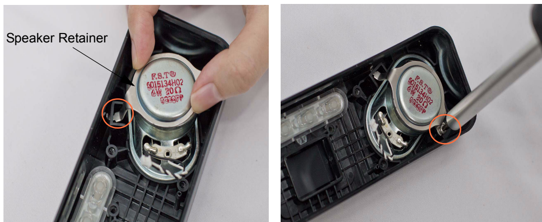
Figure 5-64 Speaker Retainer Assembly
