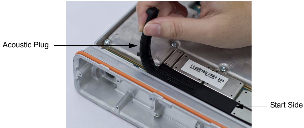
Figure 5-81 Acoustic Plug Installation
