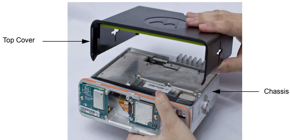
Figure 5-5 Top Cover Removal
