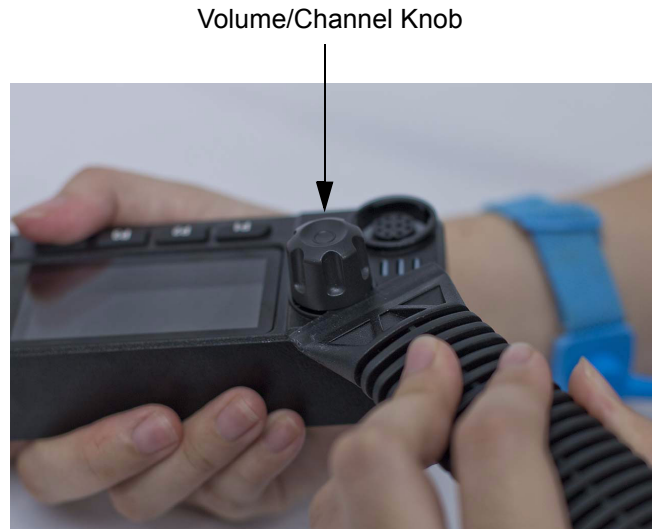
Figure 5-24 Volume/Channel Knob Removal
