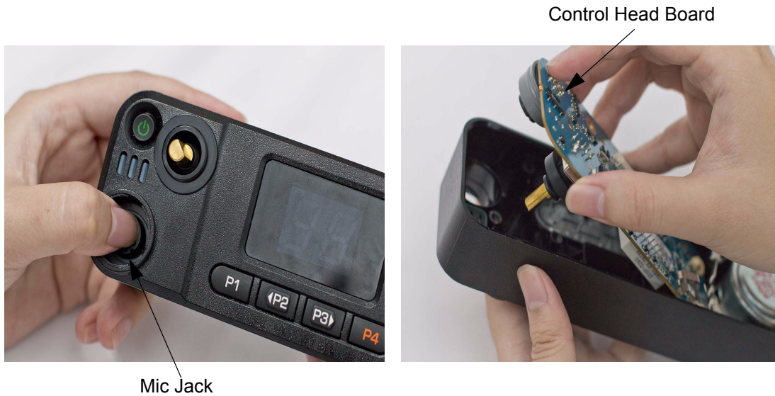
Figure 5-40 Control Head Board Removal
