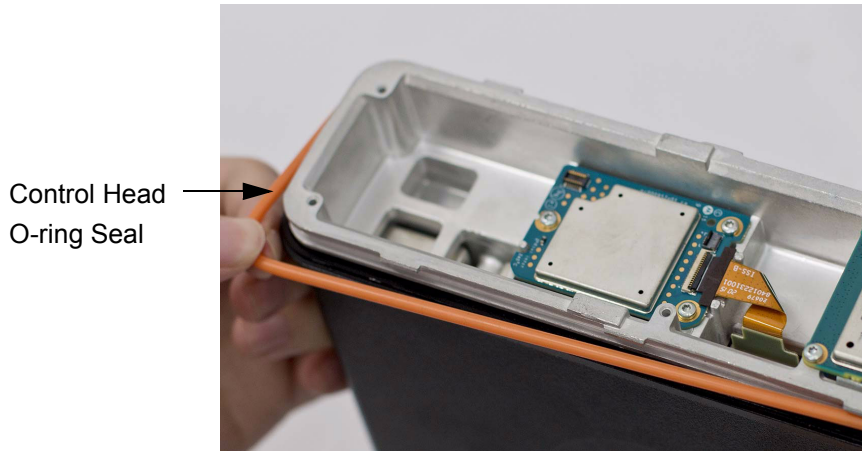
Figure 5-94 Assemble O-ring to Chassis (Image May Not Match Exact Product)
