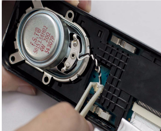
Figure 5-22 Speaker Plug Removal
