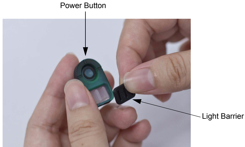
Figure 5-29 Light Barrier Removal
