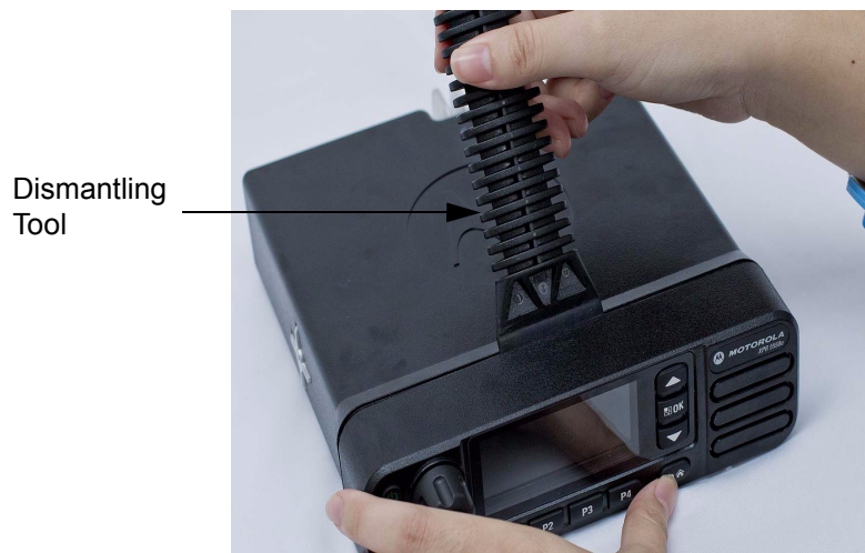
Figure 5-1 Typical Control Head Removal
