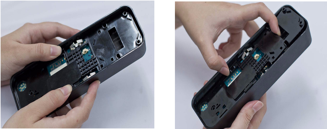
Figure 5-26 PCB Retainer Removal
