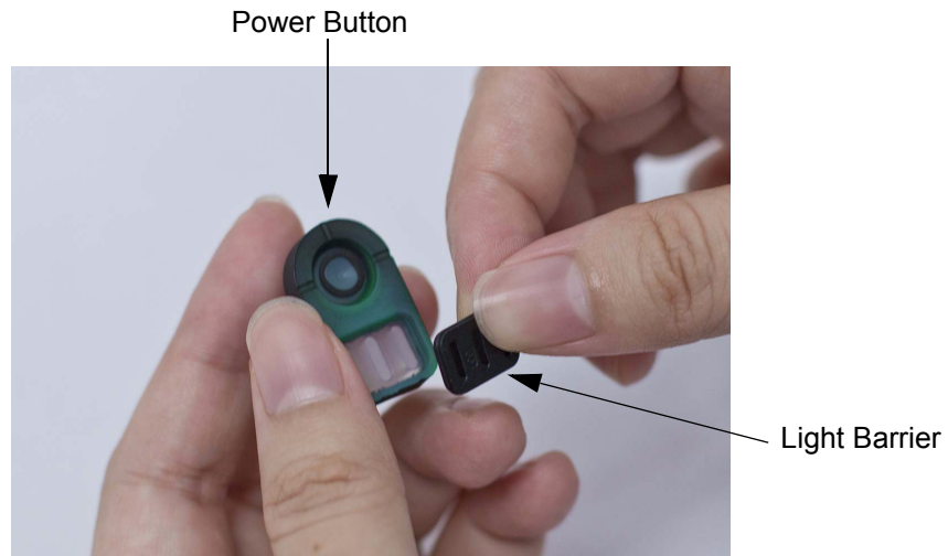
Figure 5-42 Light Barrier Removal
