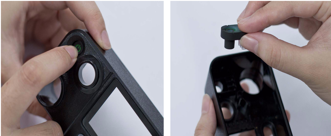
Figure 5-28 Power Button Removal
