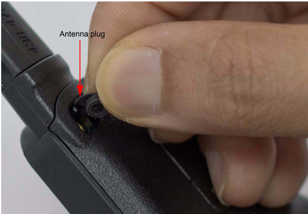
Figure 5-2. Antenna plug removal with fingers
