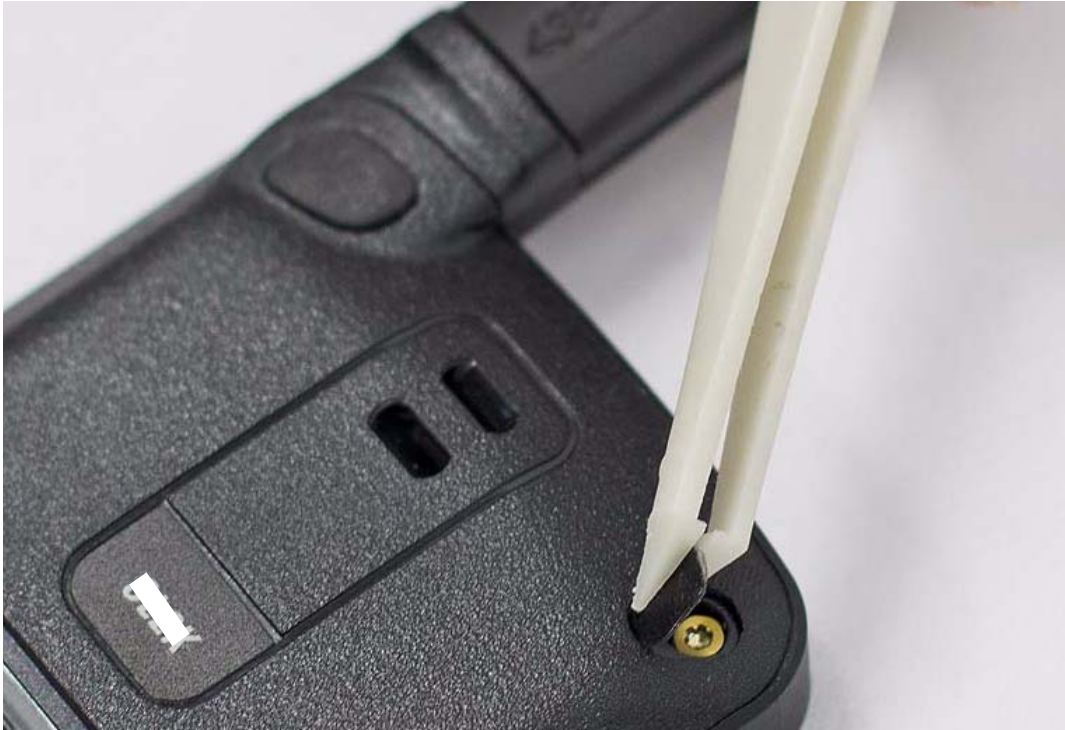
Figure 5-47. New escutcheon cover re-assembly
