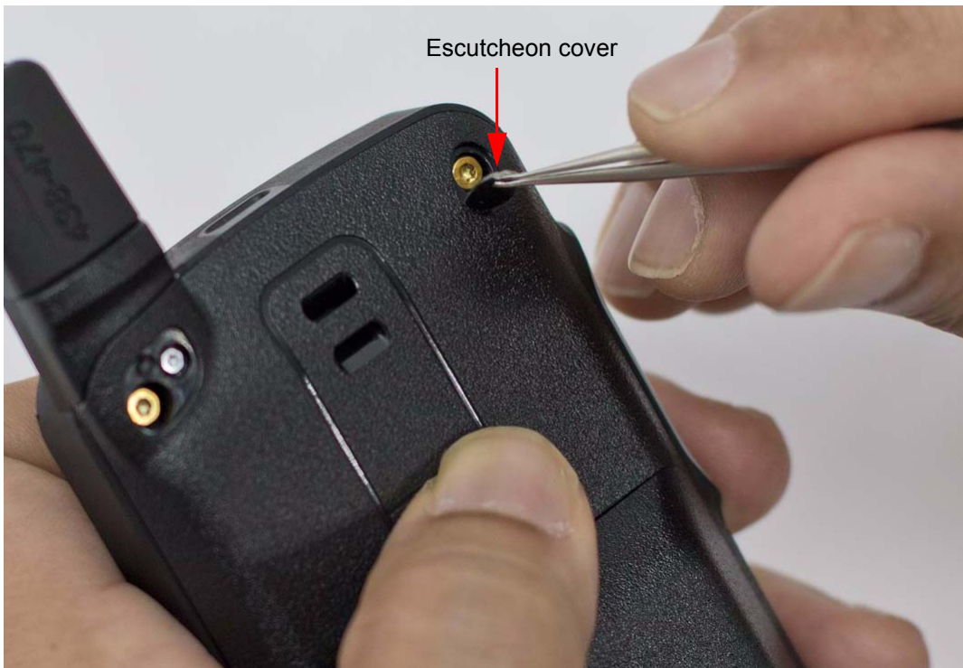
Figure 5-3. Escutcheon cover removal with tweezers
