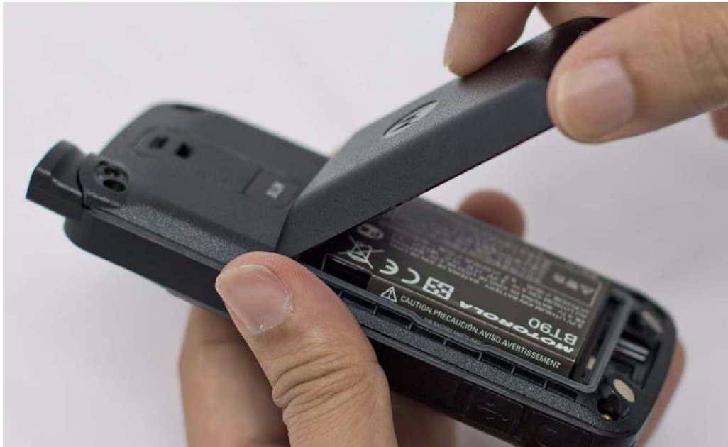
Figure 5-7. Battery door removal
