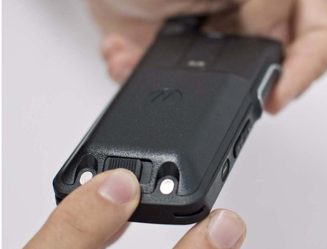
Figure 5-43. Latching battery door
