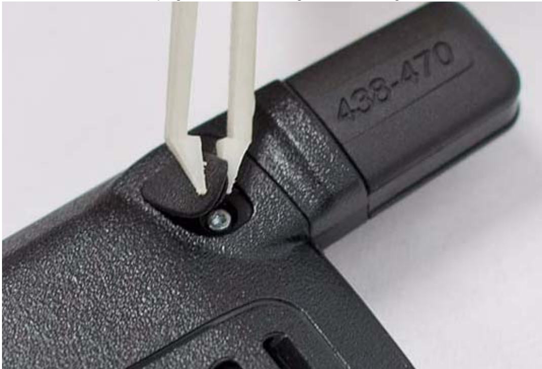
Figure 5-46. Antenna plug re-assembly
