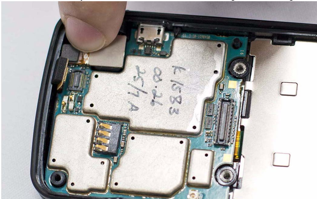
Figure 5-32. Audio jack flex connector re-assembly
