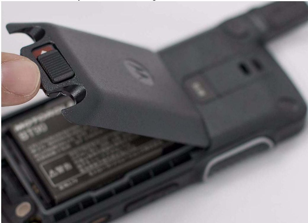
Figure 5-42. Battery door re-assembly
