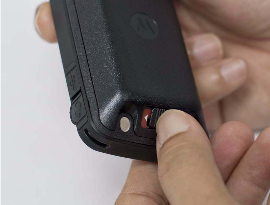
Figure 5-6. Unlatching battery door
