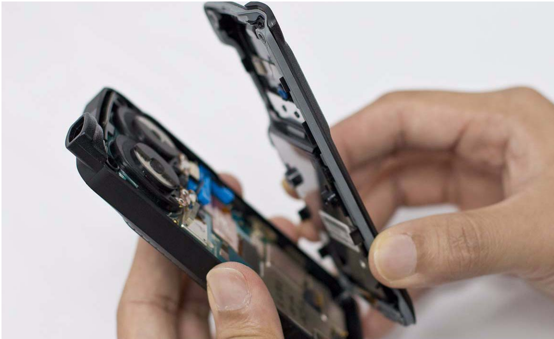
Figure 5-10. Back housing removal
