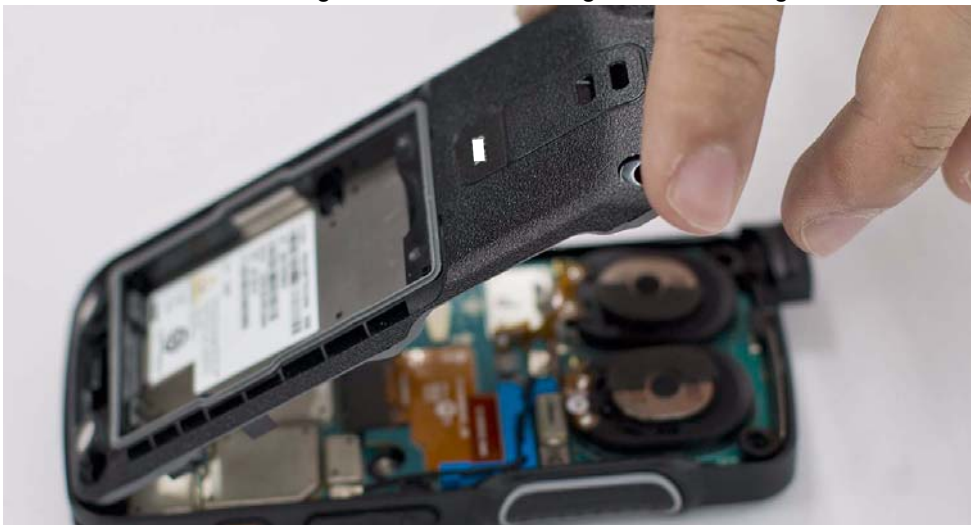
Figure 5-38. Back housing re-assembly
