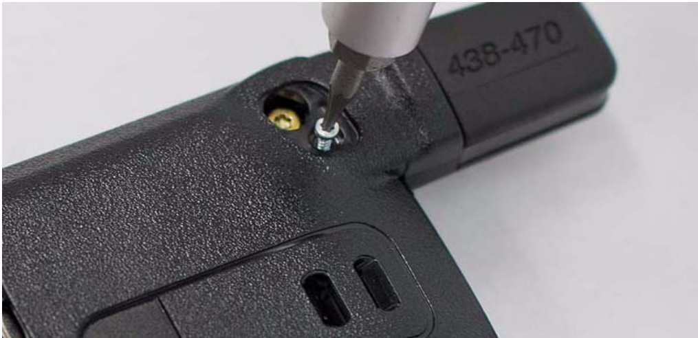
Figure 5-45. Antenna screw re-assembly
