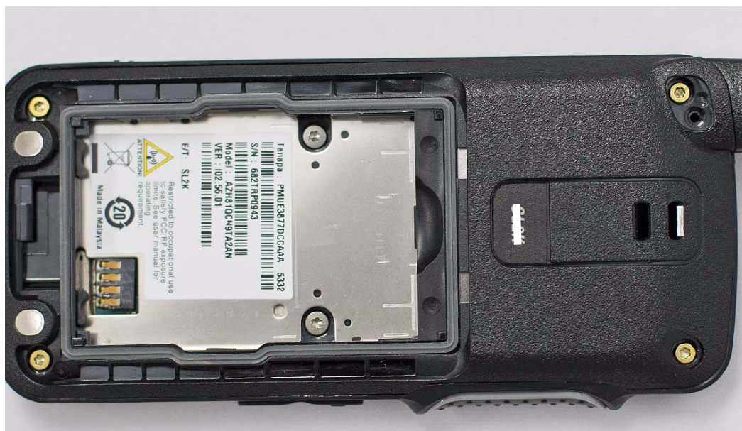
Figure 5-40. Screws re-assembly completed
