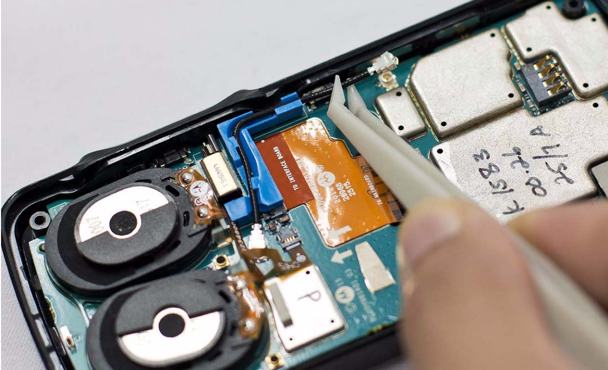
Figure 5-12. Coax cable connector disassembly
