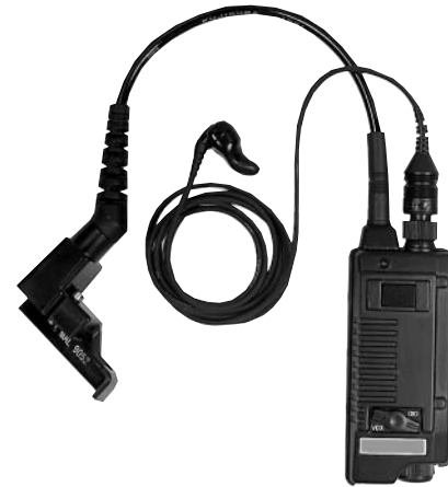
BDN6641A shown with BDN6671B interface module
