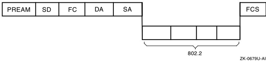
Figure F-5 illustrates the 802.2 LLC PDU and the 802.2 LLC SNAP PDU. One of these two structures is contained within the 802.3 and FDDI frame formats.
