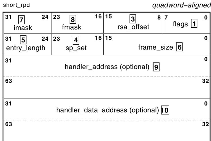
Alternate first 32-bit word for register frames
