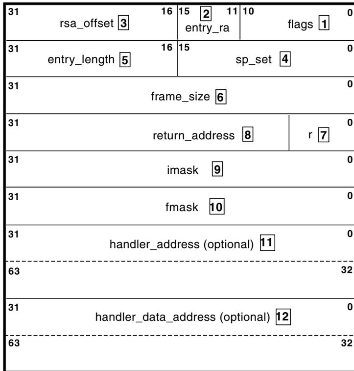
*Alternate first 32bit word for register frames*
