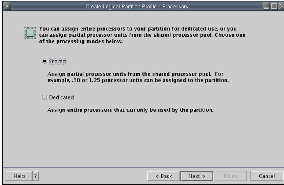
Figure 1-19 Shared processing mode for logical partition with shared processors
