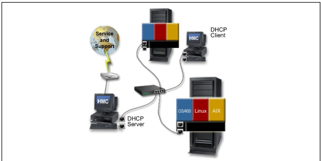
Figure 3-10 HMC with indirect network attach
